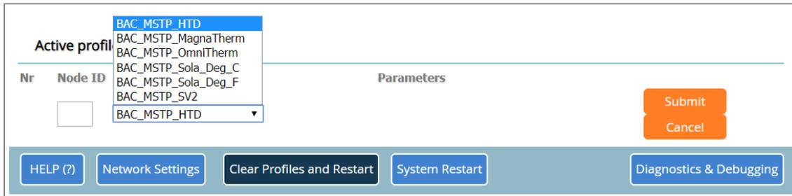
Figure 21: Web Configurator Showing Available Profile Selection
