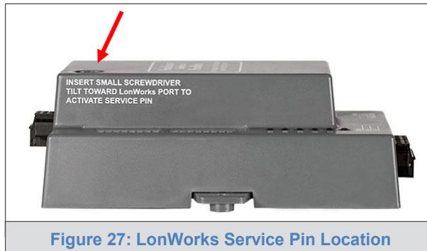
Figure 27: LonWorks Service Pin Location
