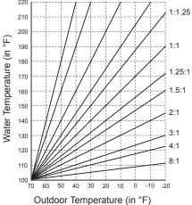
Reset Ratio is Presented as Outdoor Temp. : Water Temp. Ratio
