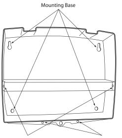
Display Mounting Screws Wiring Cover Mounting Screws
