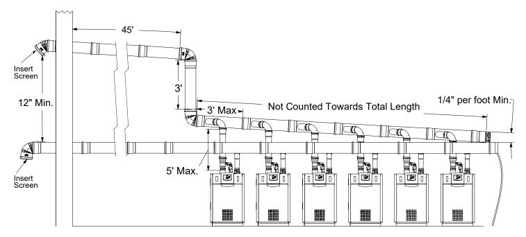
In the example system above, 6 NTH210 modulating boilers are to be installed with a common vent.
