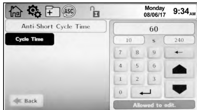
Screen 38. Anti-Short Cycle Configuration Screen
