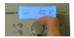
Using the Scroll/Select button locate 6:cH
