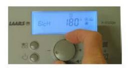
Using the Scroll/Select button locate 6:cH
