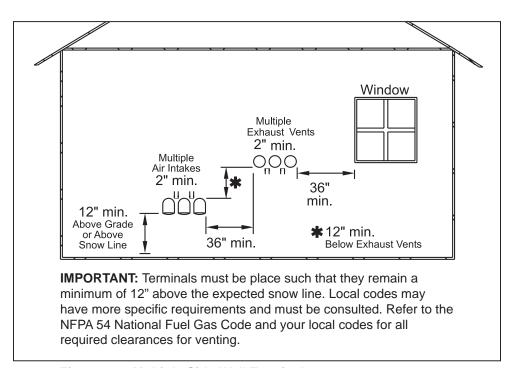
Figure 21. Multiple Side-Wall Terminals,
