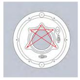
Figure 50. Torque Pattern
