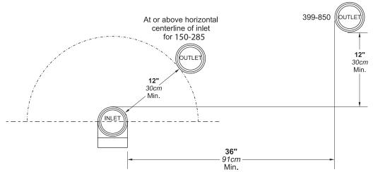
Figure 19. Minimum Venting Distance
