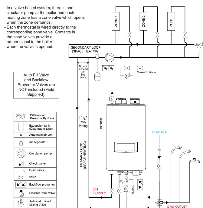
1. This piping diagram is meant to show system piping concept only. Installer is responsible for all equipment and detailing required by local codes.
