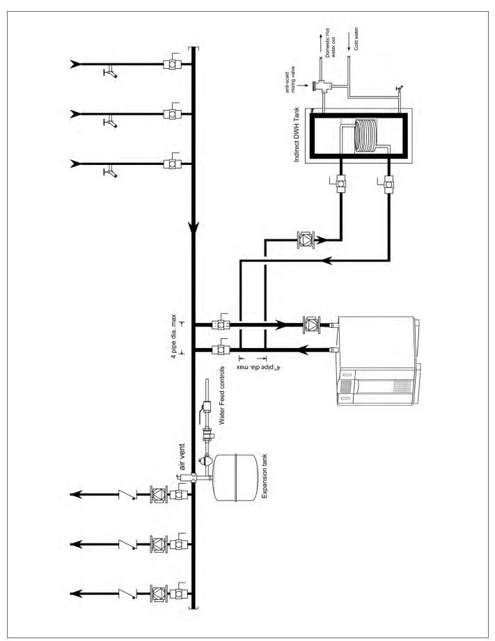
Figure 14. Hydronic Piping — Heating Zones with Indirect DHW Tank Piped with Zone Pumps The indirect DHW tank is piped directly off of the boiler.
