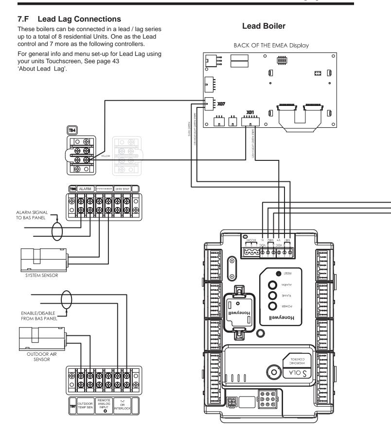
Figure 17. Wiring Diagram for Lead Lag Connections
