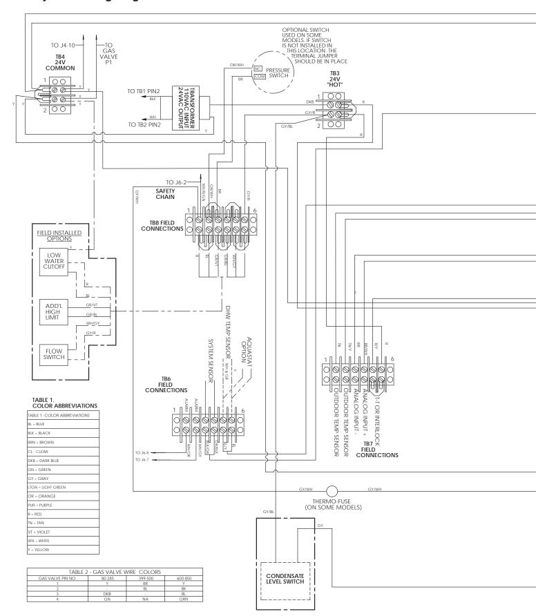
Figure 18. - Wiring Diagram, All Sizes
