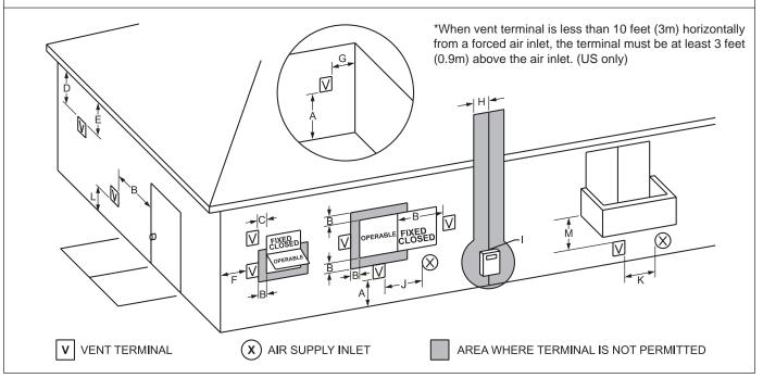
Figure 7. - Combustion Air and Vent Through Side Wall
