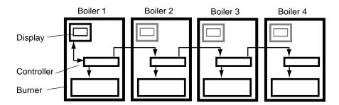
**Figure 33.** "Lead Lag" Operation in a System with Four Boilers. Note - the Displays on Boilers 2 thru 4 will display information pertaining only to that specific boiler.
