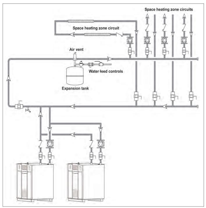
Figure 11. Hydronic Piping — Multiple Boilers, Zoning with Circulators
