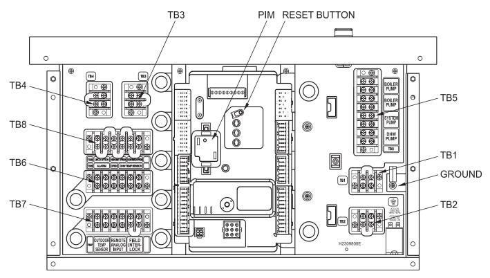
Figure 30. - Control Panel Layout
