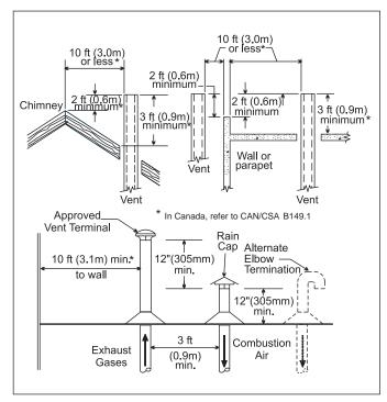
Figure 4. - Combustion Air and Vent Through Roof
