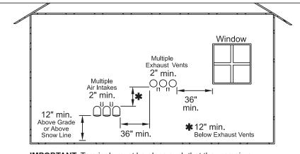
**IMPORTANT:** Terminals must be place such that they remain a minimum of 12" above the expected snow line. Local codes may have more specific requirements and must be consulted. Refer to the NFPA 54 National Fuel Gas Code and your local codes for all required clearances for venting.
