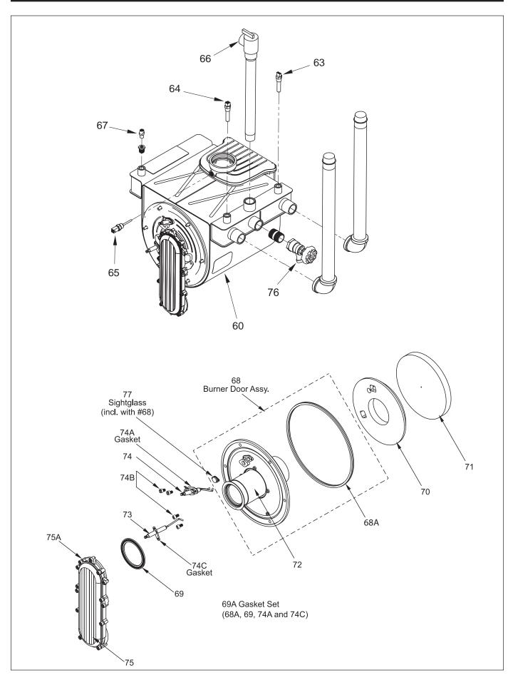
Figure 44. - Heat Exchanger Components
