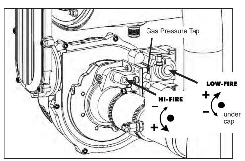
Figure 36. - Unit Gas Valve 80 - 210 Mbtu
