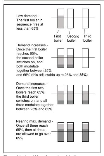
Figure 34. Lead / Lag Operation, 3 boilers.
