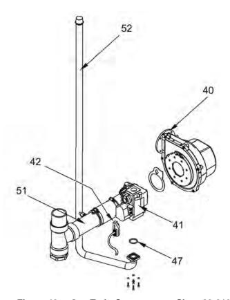
Figure 42. - Gas Train Components, Sizes 80-210
