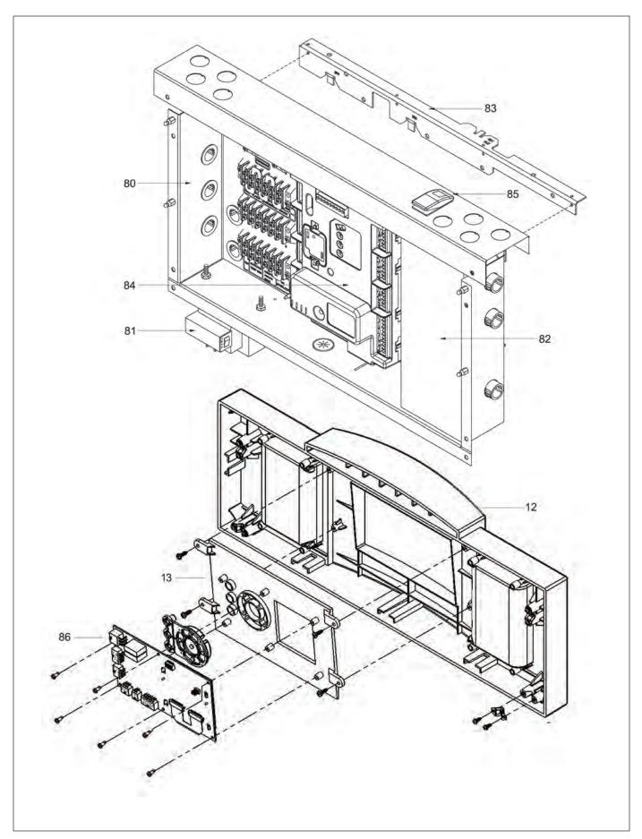
Figure 45. - Electrical Components
