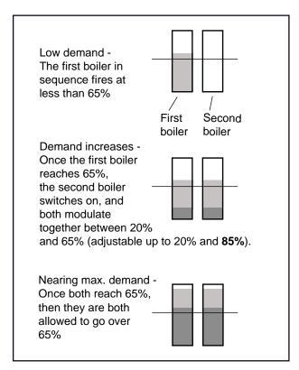
Figure 32. Lead / Lag Operation, 2 boilers.
