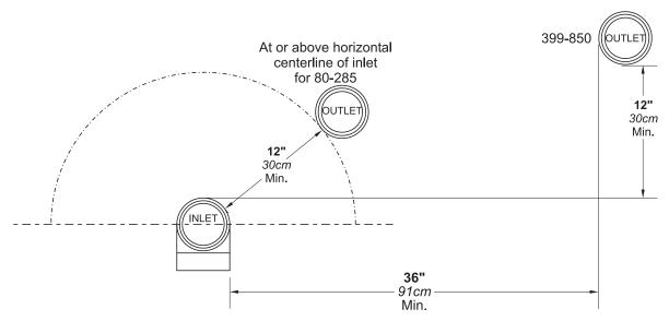
Figure 8. - Minimum Venting Distance
