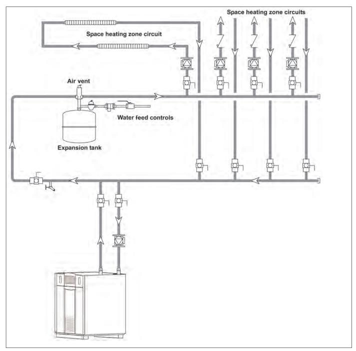
Figure 9. Hydronic Piping — Single Boiler, Zoning with Circulators
