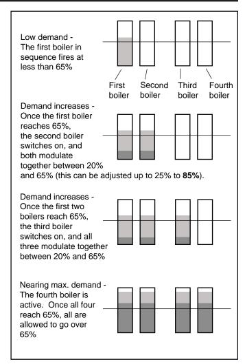
Figure 35. Lead / Lag Operation, 4 or more boilers.
