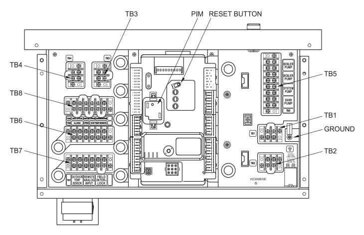
Figure 16. Control Panel Layout
