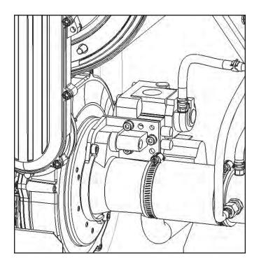
The Gas Valve in the 80 thru 210 is at the front of the unit and can be reached after the front panel is pulled forward and then off.
