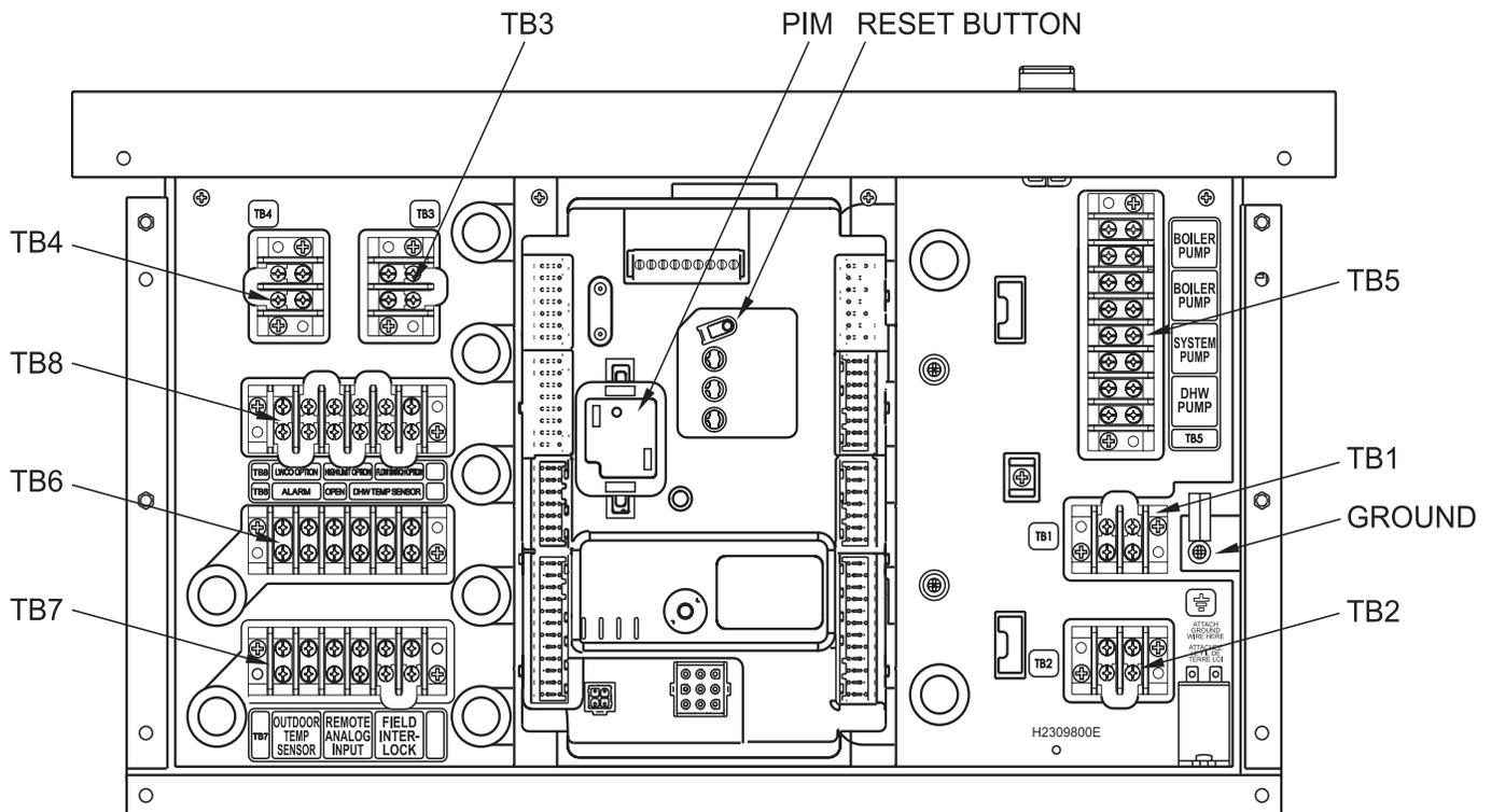
Figure 31. - Control Panel Layout
