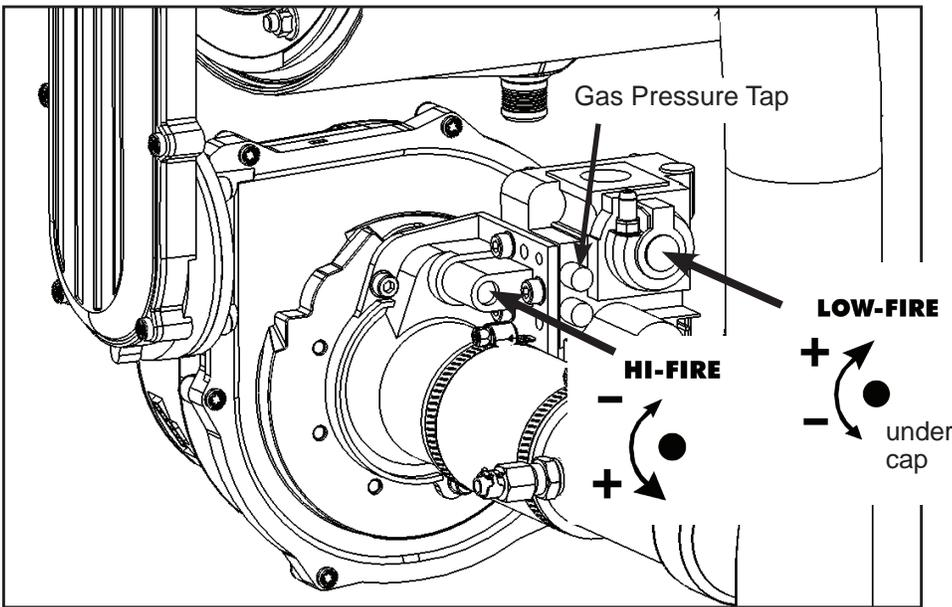
**Figure 36. - NeoTherm Gas Valve 80 - 210 Mbtu**
