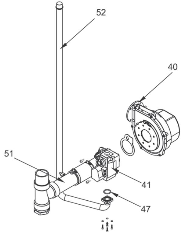
**Figure 41. - Gas Train Components, Sizes 80-210**
