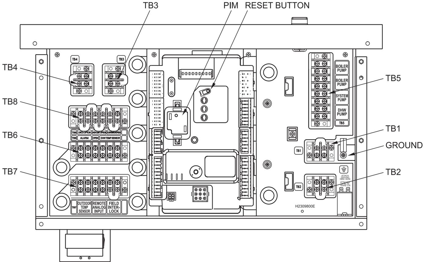
Figure 16. - Control Panel Layout
