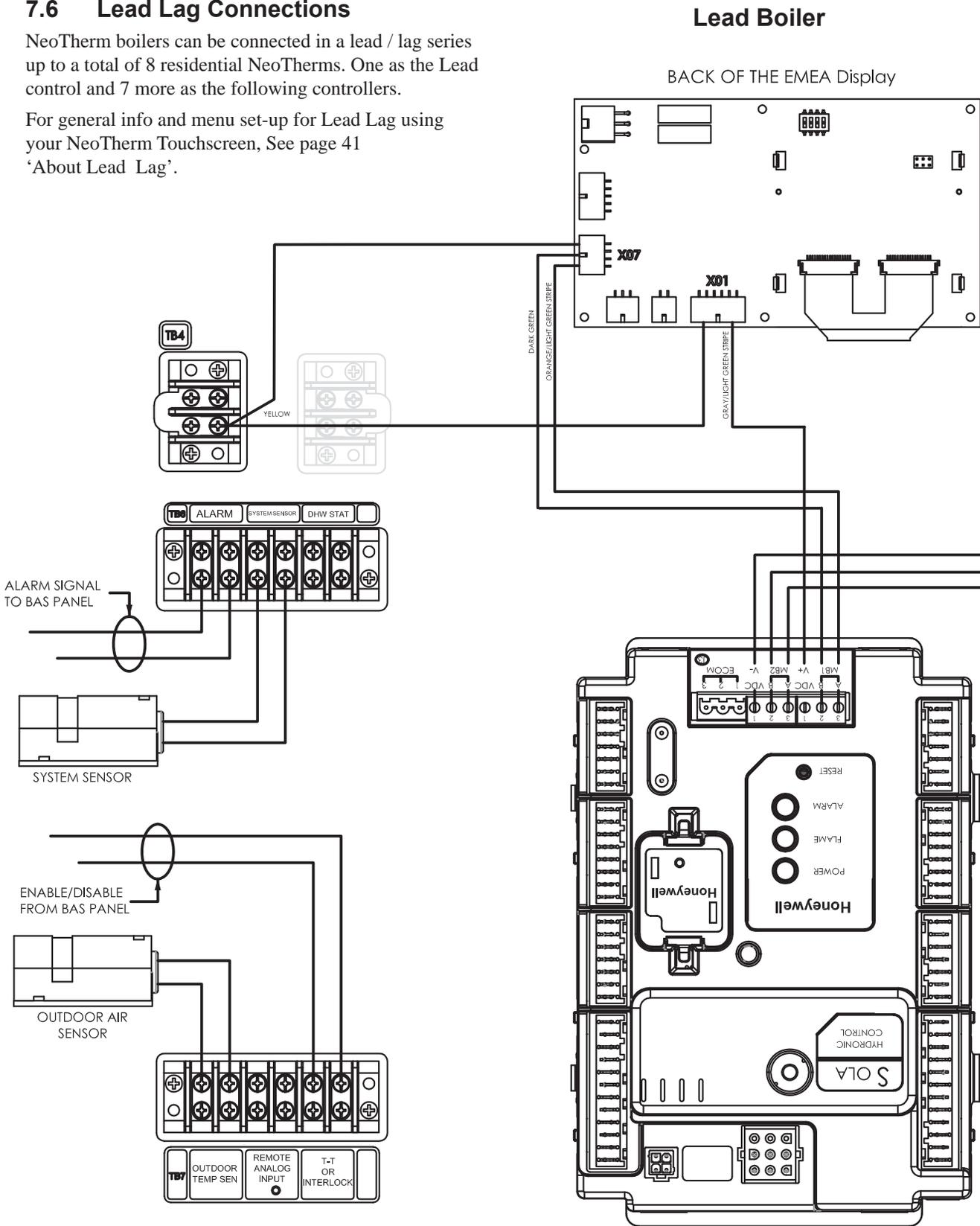
Figure 17. Wiring Diagram for Lead Lag Connections
