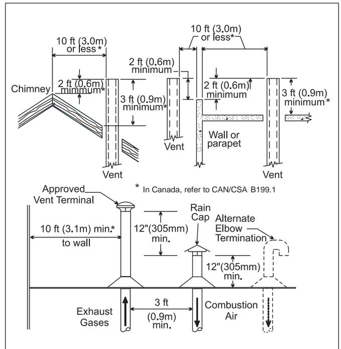
**Figure 4. - Combustion Air and Vent Through Roof**
