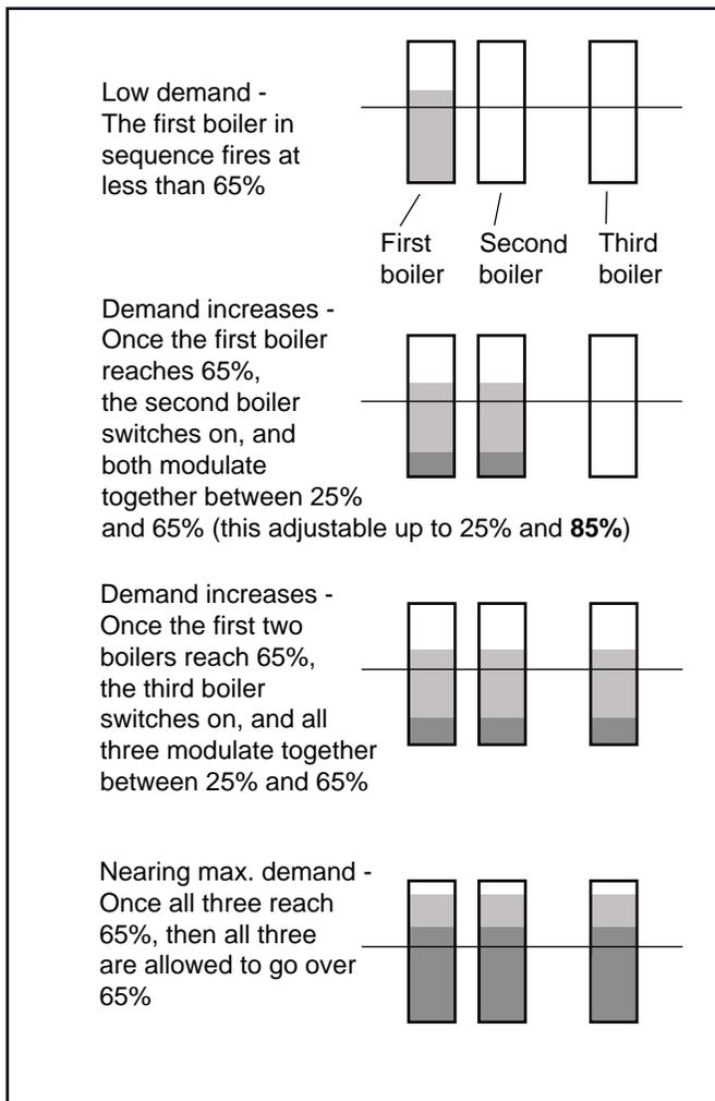
**Figure 34. - Lead / Lag Operation, 3 boilers.**
