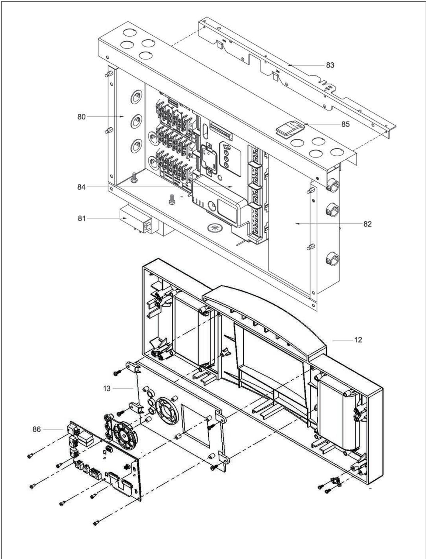
**Figure 44. - Electrical Components**
