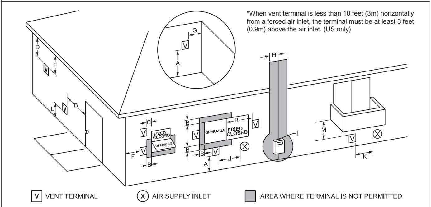
**Figure 6. - Combustion Air and Vent Through Side Wall**
