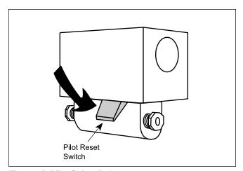
Figure 15. Pilot Safety Relay.
