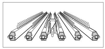
Figure 16. Main Burner Flame Pattern.
