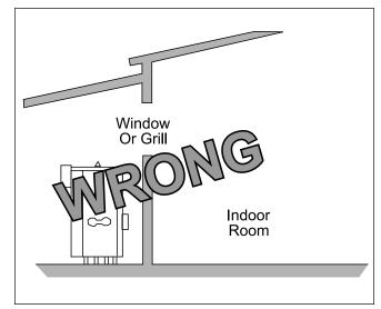
Figure 10. Incorrect Outdoor Installation.
