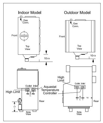
Figure 1. Boiler Configuration.
