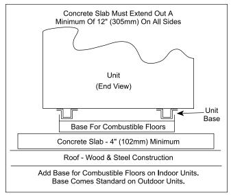
Figure 5. Typical Boiler Installation on Concrete Slab.
