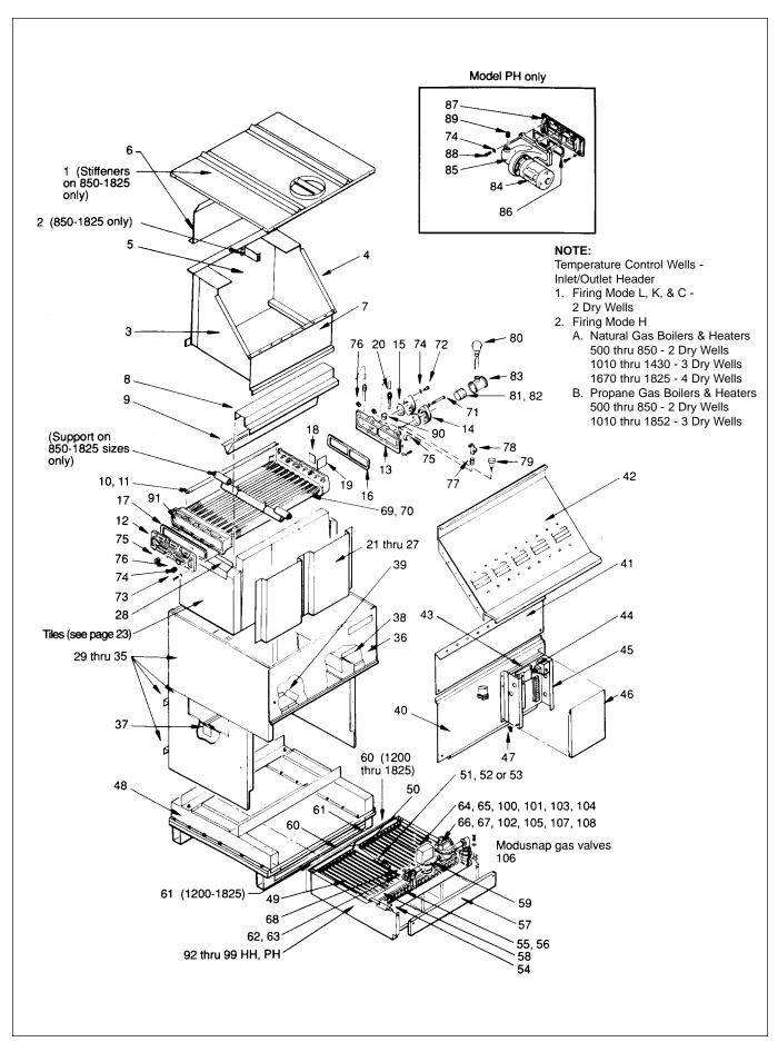
Figure 19. Parts Identification.
