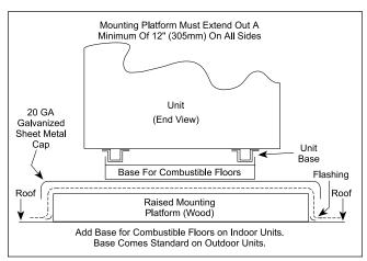
Figure 6. Typical Boiler Installation on Raised Platform (Wood).
