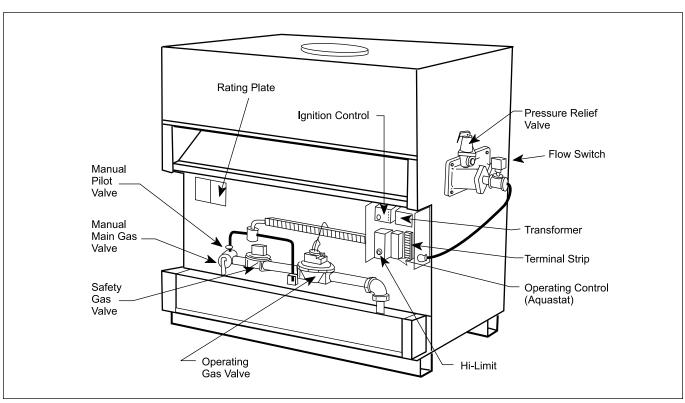
Figure 13. Typical Controls Locations.
