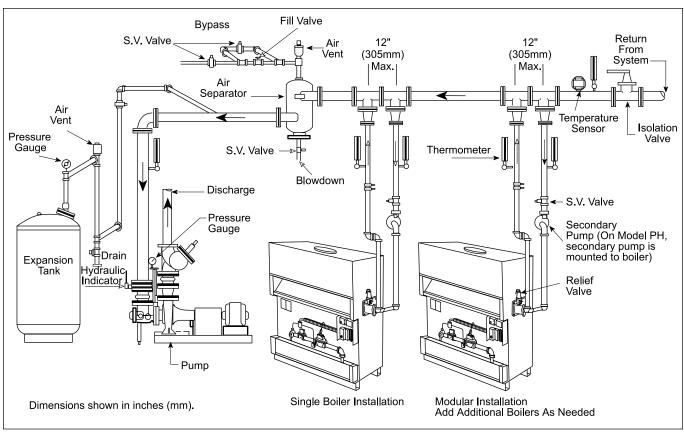
Figure 2. Typical Schematic for a Primary-Secondary System.
