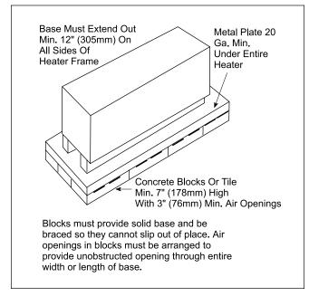
Figure 8. Installation on Concrete Blocks or Tile.
