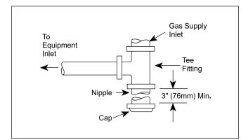
Figure 11. T-Fitting Sediment Trap Installation.
