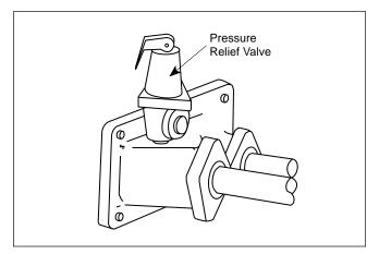
Figure 12. Pressure Relief Valve Location.
