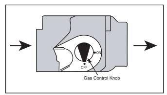
Figure 1 - Gas Control for Automatic Ignition System (JVS)
