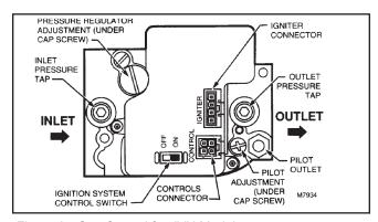
Figure 2 - Gas Control for JVH Models
