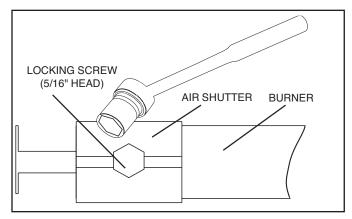
Figure 5 - Removing the Air Shutter Locking Screw
