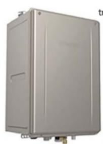
triggers recirculation-loop activation. Available with inputs of 165,000 Btu per hour (NRCR92-DV) and 199,900 Btu/ hr. (NRCR111-DV). Both Energy Star-rated models carry a UEF of 0.97. Venting involves 2" or 3" PVC or CPVC pipe, with vent runs up to 65' for 2" pipe and up to 150 ft. for 3". The NRCR92-DV has a capacity range of 0.5 to 9.2
