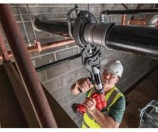
Extended 32kN applications to press 2½" to 4" carbon steel. The tool is compatible with the RIDGID full line of Standard 32kN Press Tool accessories, including the StrutSlayr™ Strut Shear Head, Press Snap™ Soil Pipe Cutter and all MegaPress jaws.
