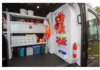
yet lightweight at just 55 lbs. The accessory panels are designed to accompany the WEATHER GUARD REDZONE accessories, but also offer standard threaded inserts for off-the-shelf attachments. It is custom-designed for the most popular commercial vans.
