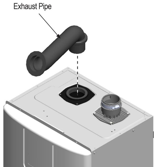
2. Insert the VCK Exhaust Adapter and secure the front 2 screws (re-use the 2 screws that were removed in Step 1)
