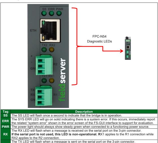
Figure 44: Diagnostic LEDs
