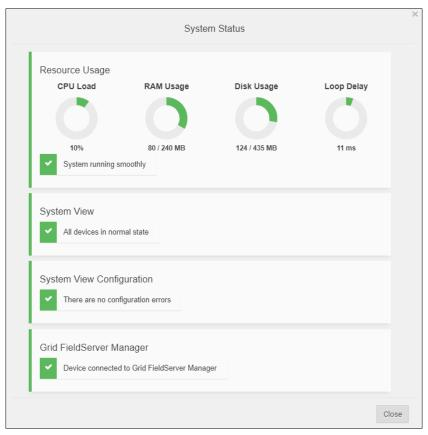
NOTE: If it was selected to opt out of the FieldServer Manager (Figure 24), the Grid FieldServer Manager status will not show in the System Status window. This means the status will show as green even if the gateway is not connected to the FieldServer Manager.
