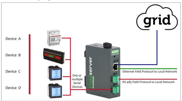
The ProtoNode can connect with the MSA Grid – FieldServer Manager. The FieldServer Manager allows technicians, the OEM's support team and MSA Safety's support team to remotely connect to the ProtoNode. The FieldServer Manager provides the following capabilities for any registered devices in the field:
