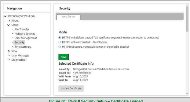
Figure 50: FS-GUI Security Setup - Certificate Loaded
