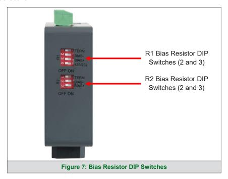
To enable Bias Resistors, move both the BIAS- and BIAS+ dip switches to the right as shown in Figure 7.
