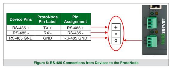
Wiring Field Port to RS-485 Serial Network
