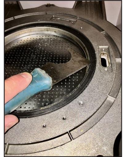
Step 12. Pry or pull the burner from the lower burner plate. Use caution to avoid bending the burner flange.
