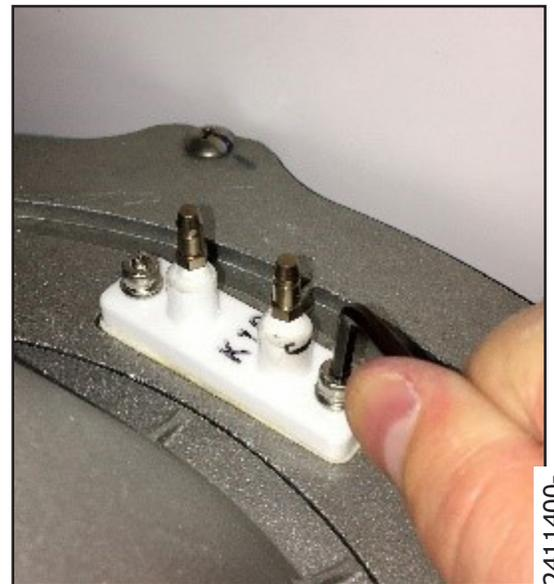
Step 9. Remove the four mounting screws from the upper burner case and separate it from the lower burner case. The burner gasket may cause the upper burner case to stick.
