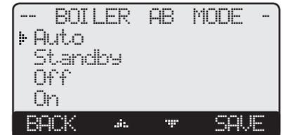
**Auto** - The S8 will control the unit's operation to maintain the desired Set Point. Only units set to Auto can be Lead.
