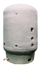
Laars Stratified Storage Tanks for Heat Pump Systems are designed specifically to optimize installed heat pump system performance. Tanks are offered with red oxide primer and a 2-1/4" high-density polyurethane foam and acrylic top coat for increased energy savings. Typical tank configurations include multiple 340-gallon, 500-gallon or multiple 1000-gallon tanks that are piped to maximize temperature stratification.
