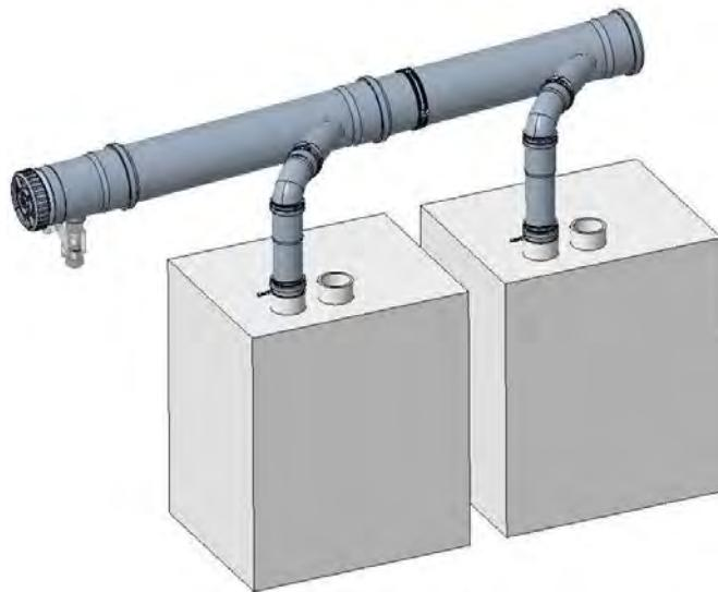
Note: Canadian installations require two non-return-valve kits D2027800 to be used in conjunction with this kit (one for each boiler). Use in U.S. installations is optional.
