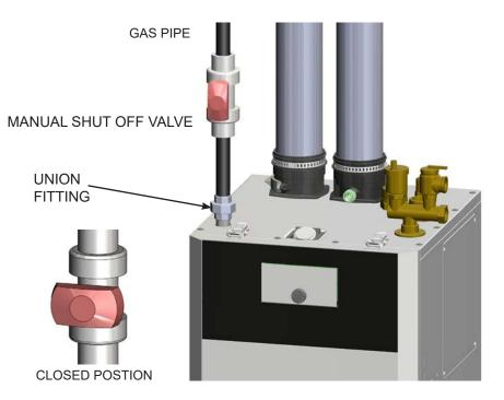
Gas Line Shut Off Valve Detail
