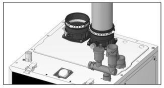
2" pipe connected, using an adapter
