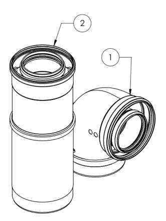
**7)** Add the 810005865, (#1), 3X5 Concentric 90° elbow from the FT3004 Kit until it bottoms out. Adjust the length of the telescopic section as required.
