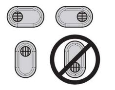
Low profile terminations must be installed in the proper orientation.
