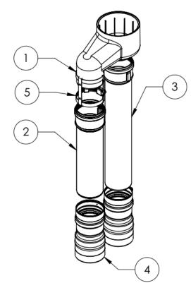
**5)** Insert the, 17.75" Straight Length, plain end PP pipe through the top of the , (#1), concentric PP adaptor. Do not connect it to the FT boiler or FT3001 Elbow, if used, at this point.
