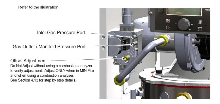
The Maximum and Minimum gas line pressures must be at Max Fire operation.
