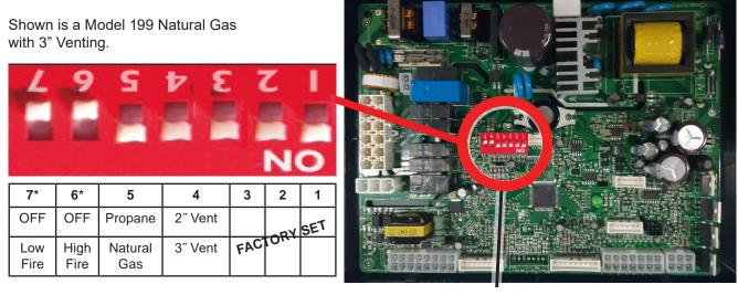
\*DIP Switches #7 and #6 are Maximum and Minimum fire test Switches which are used only when setting up combustion (See Section 4.13). These switches should only be in the ON position during either High or Low fire testing. When finished testing, ensure both of these switches are in the OFF position.
