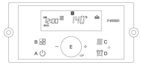
**To change Storage Mode Temp,** First turn OFF the power to the Control Display. Then Press and Hold Button B **H** to get into the Installer Mode.
