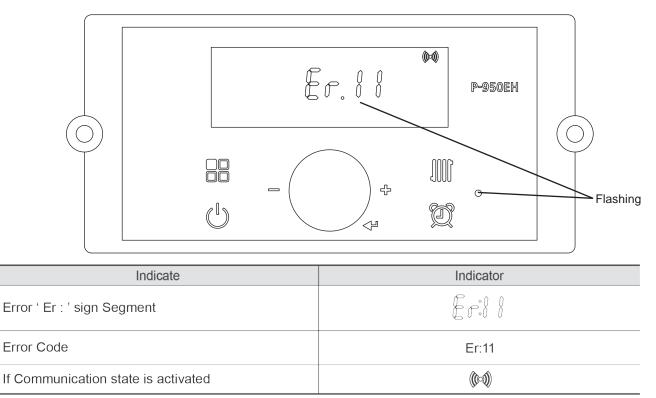
NOTE: When communication between the Control Display and the main controller is lost, the will not be displayed.
