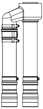
**8)** Ensure that the 12" pipe is bottomed out in the Concentric Adaptor, (#1), and install the, (#5), Clamp and tighten both ends.
