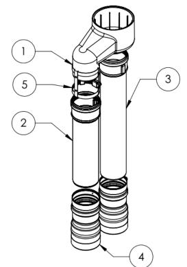
aligned with the Vent socket on the FT Boiler. Slide the 17.75" pipe down through the stainless steel to PP adapter and connect it to the adapter on the FT boiler's Vent connection. Ensure that item #3 bottoms out and tighten the clamp.
