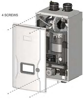
To remove the cover, unthread the 4 phillips head screws. Keep the screws in a safe place for re-application of cover. This is typical for all models of the FT Series wall.
