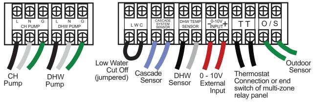
DHW and CH pump terminals for external pump are live 120V limited to 2.0 A. They operate respective to an external call (e.g T-T) for heat.
