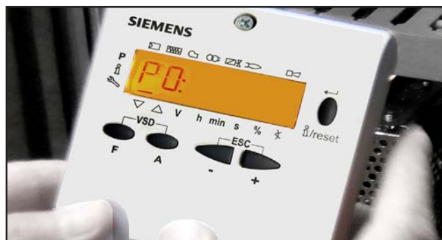
Figure 50. AZL Control (Siemens hand-held controller)
