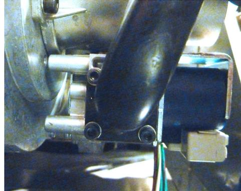
Fig. C5-6 - Four mounting screws for the gas inlet pipe (viewed from below)
