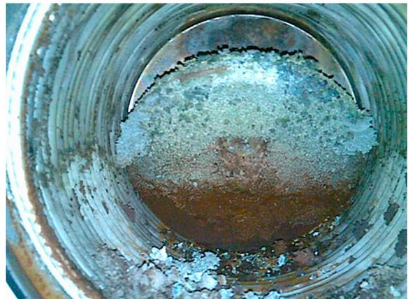
Fig. C5-13 - Very dirty heat exchanger
