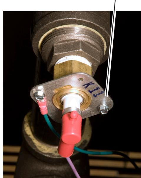
Fig. B6-1 - Removing the probe wires
