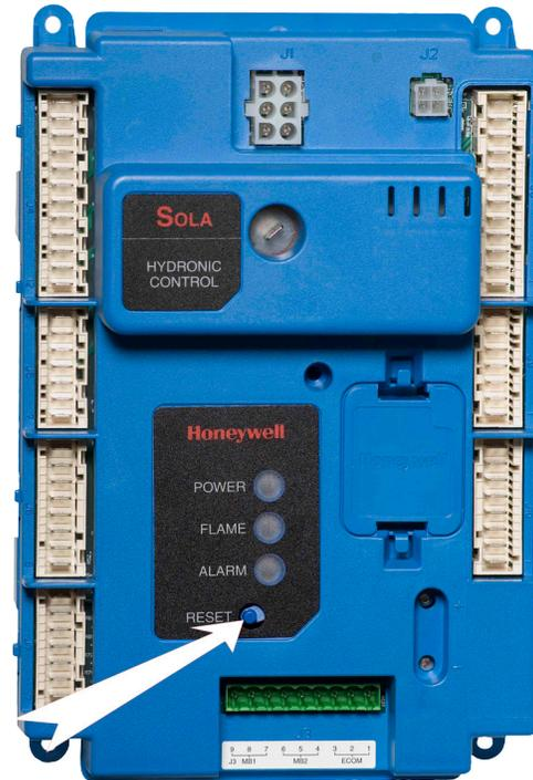
Fig. D6-1 – Resetting the SOLA controller
