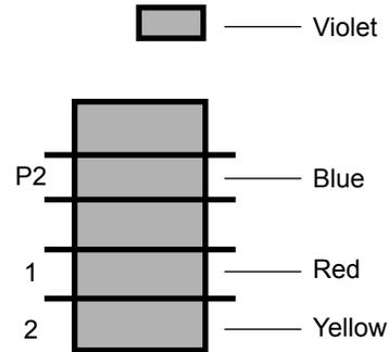
Fig. B6-3 - Connections to low water cutoff control
