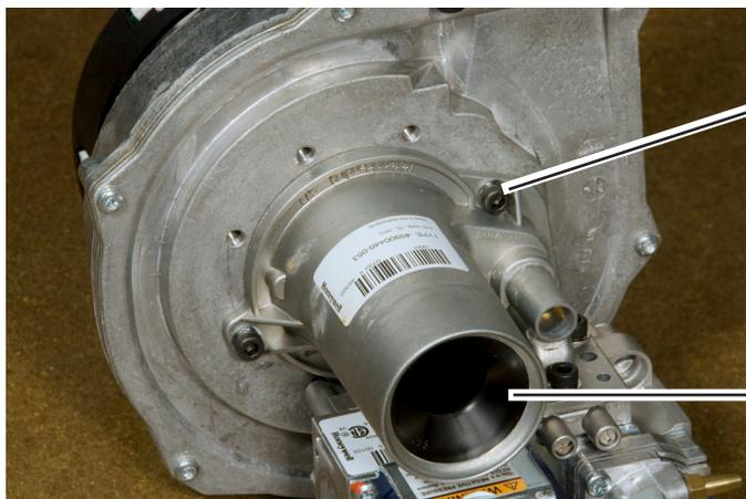
Fig. B19-9 - Removing Venturi and gas valve
