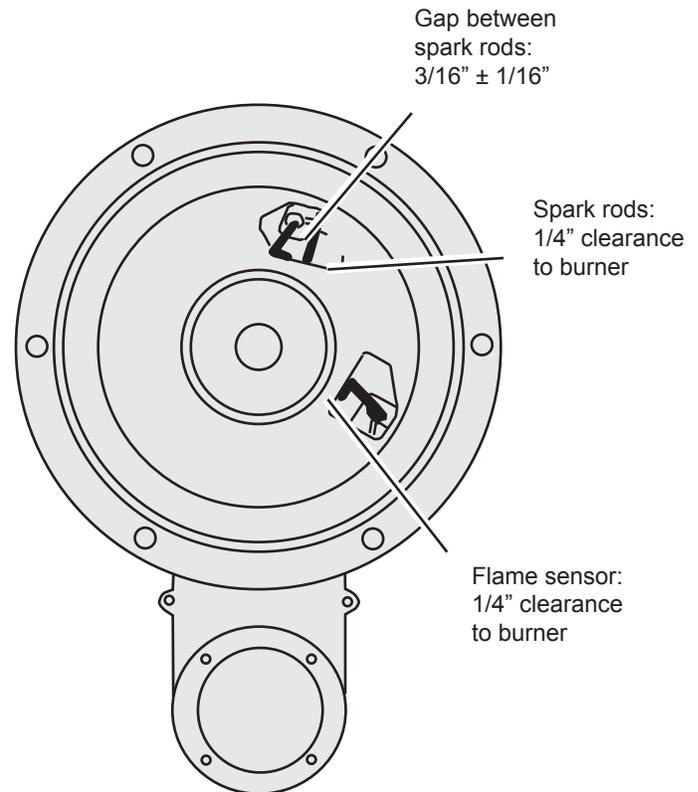
Fig. B32-2 - Correct setting for spark gap
