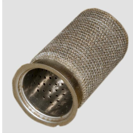
Fig. C5-9 - Burner can removed
