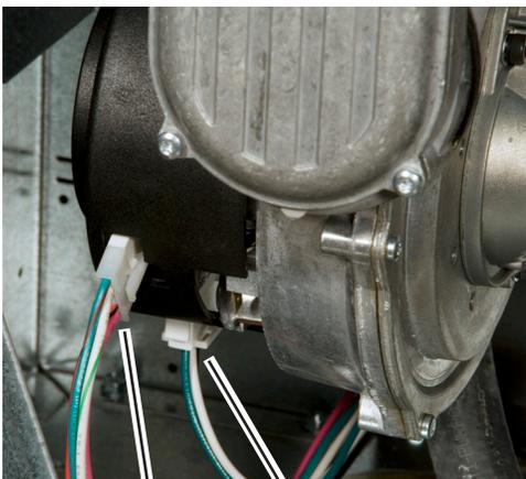
*Fig. C5-4 - Wiring connections for blower*
