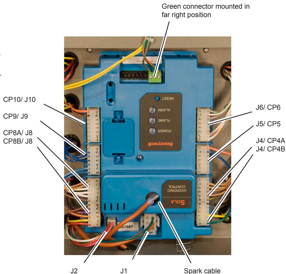
Fig. D9-2 - Connectors on the SOLA controller
