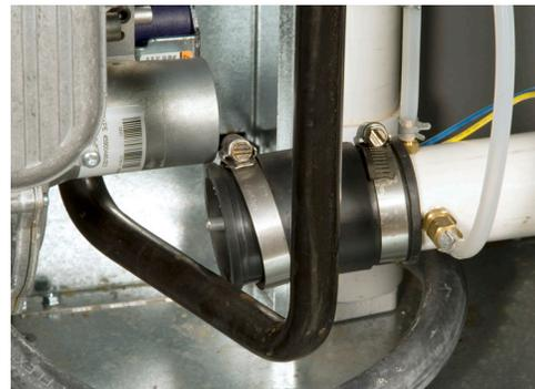
Fig. B11-5 - Loosen the left end of the rubber hose
