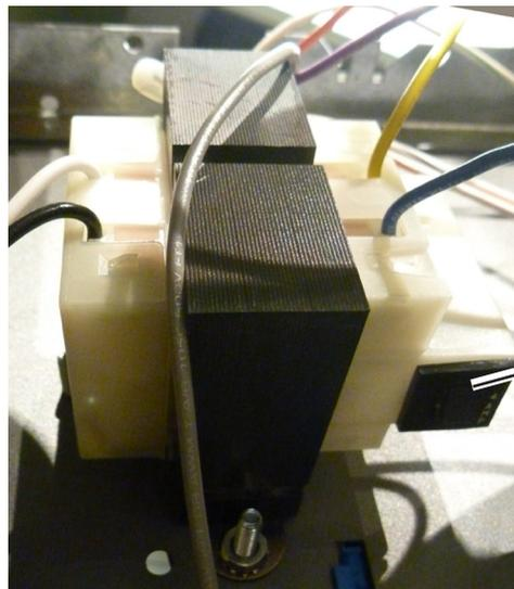
*Fig. B30-2 - Reset switch on bottom of transformer (viewed from below)*
