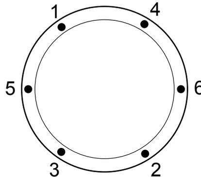
Fig. C5-16 - Tightening sequence for nuts on front cover
