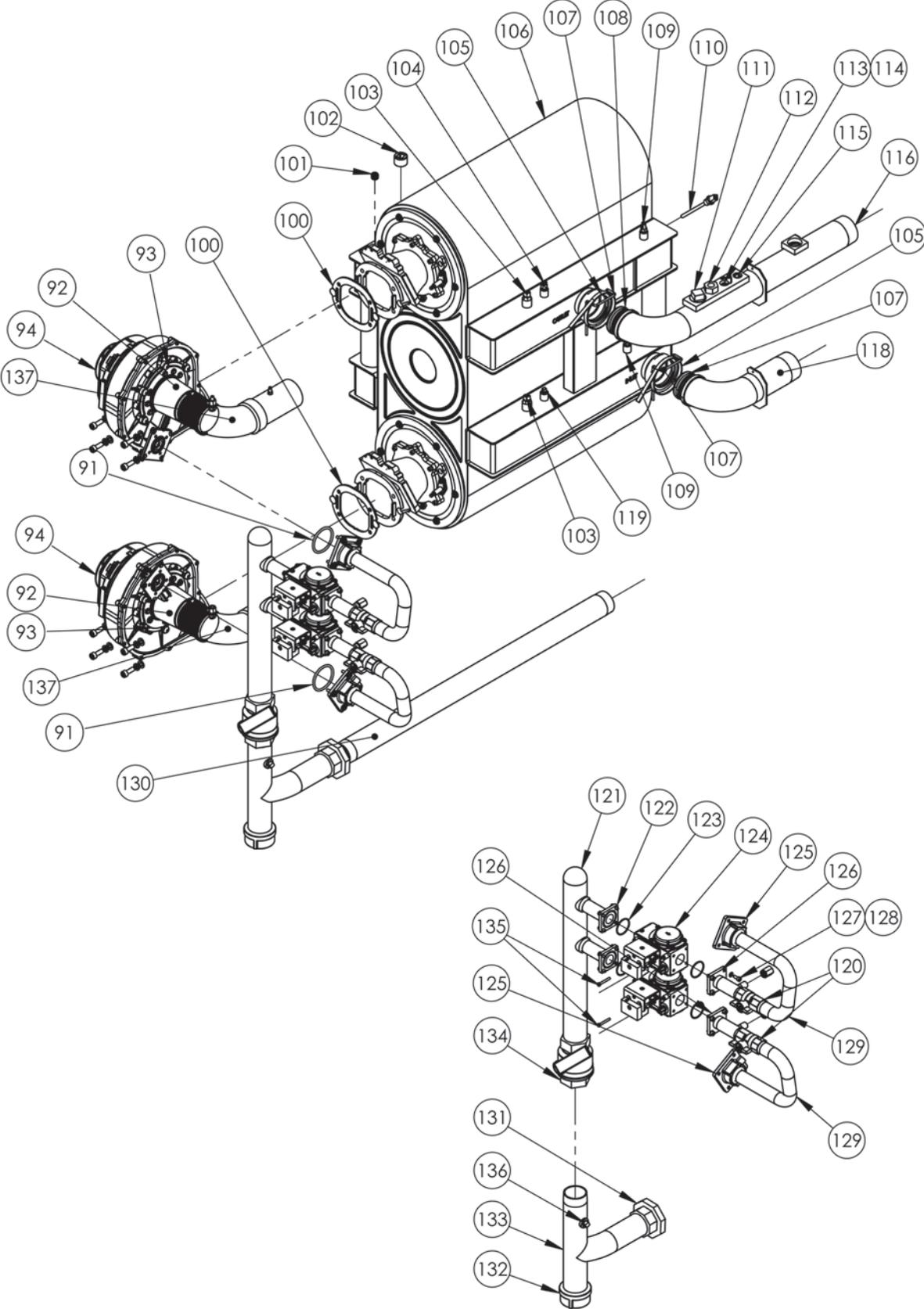
Fig. 145 - Burners and Combustion Chamber
