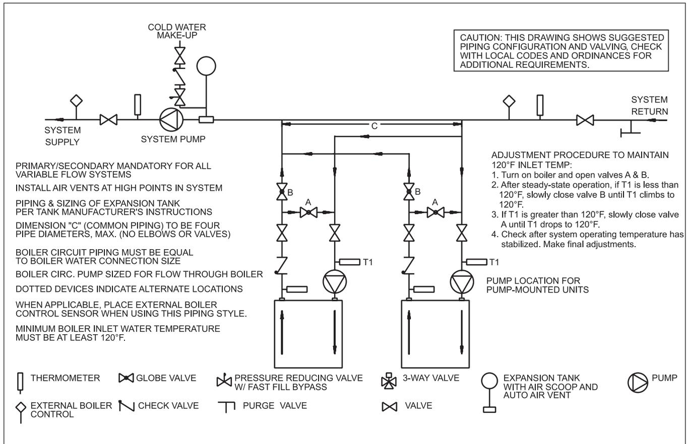
Figure 9. Hydraulic Piping — Primary-Secondary, Reverse-Return, Low Temperature.
