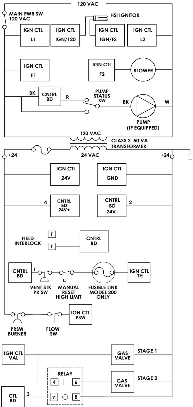
Figure 14. Logic Diagram, Hydronic Boiler
