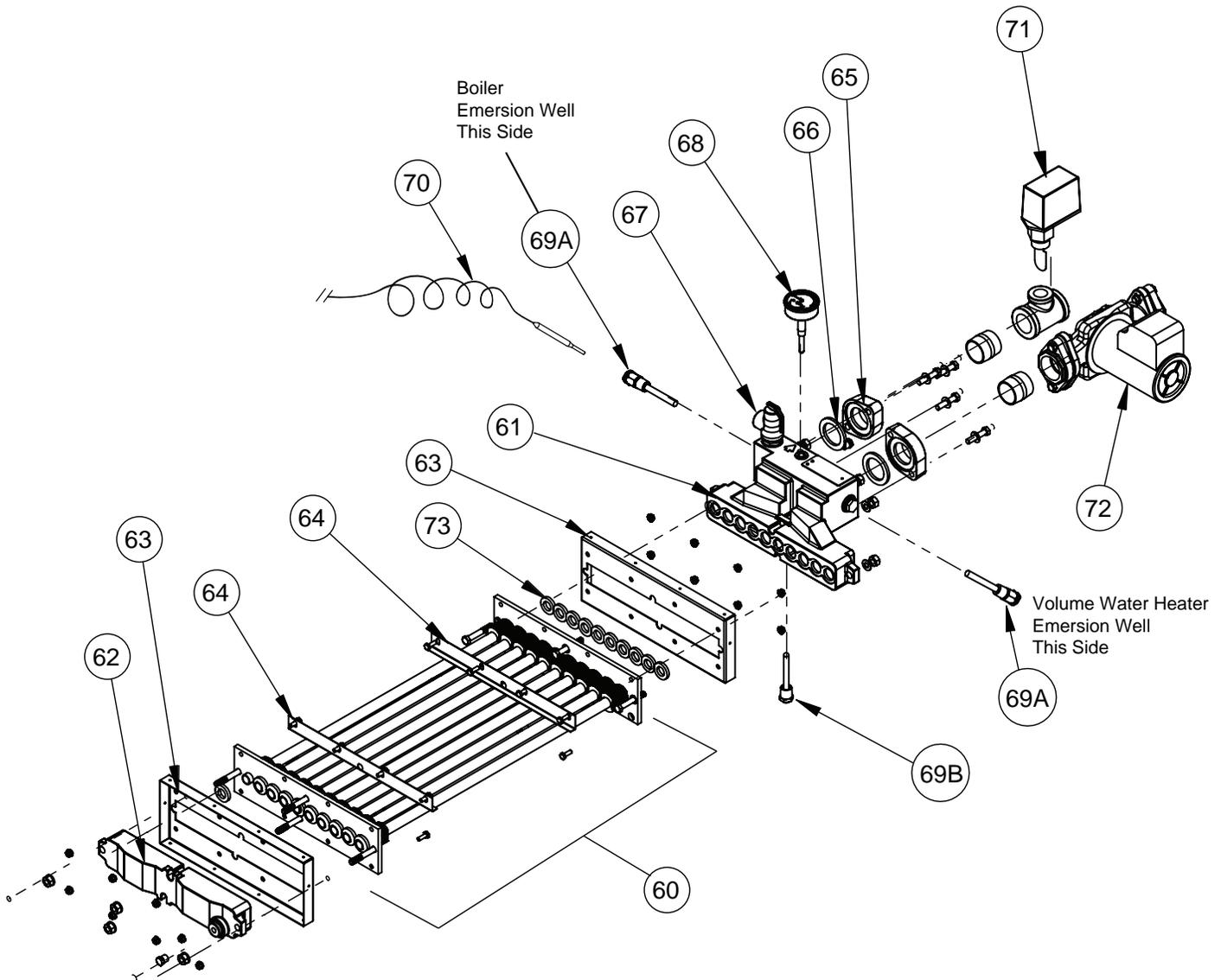
Figure 21. Heat Exchanger Components.
