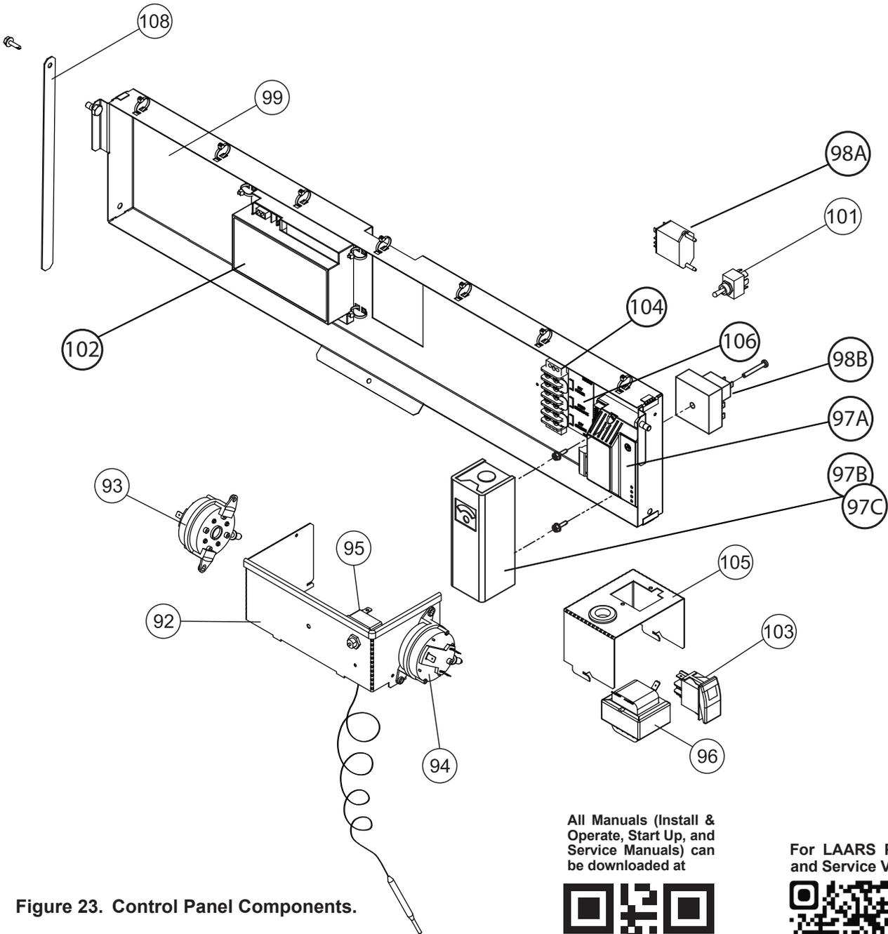
Figure 23. Control Panel Components.
