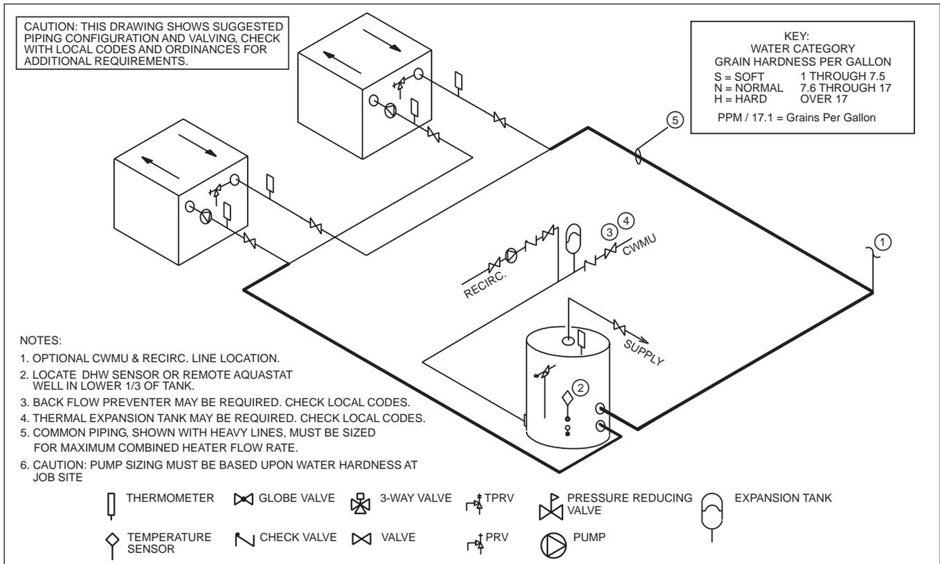
**Figure 11. Water Heater Piping — Multiple Heaters, One Tank.**
