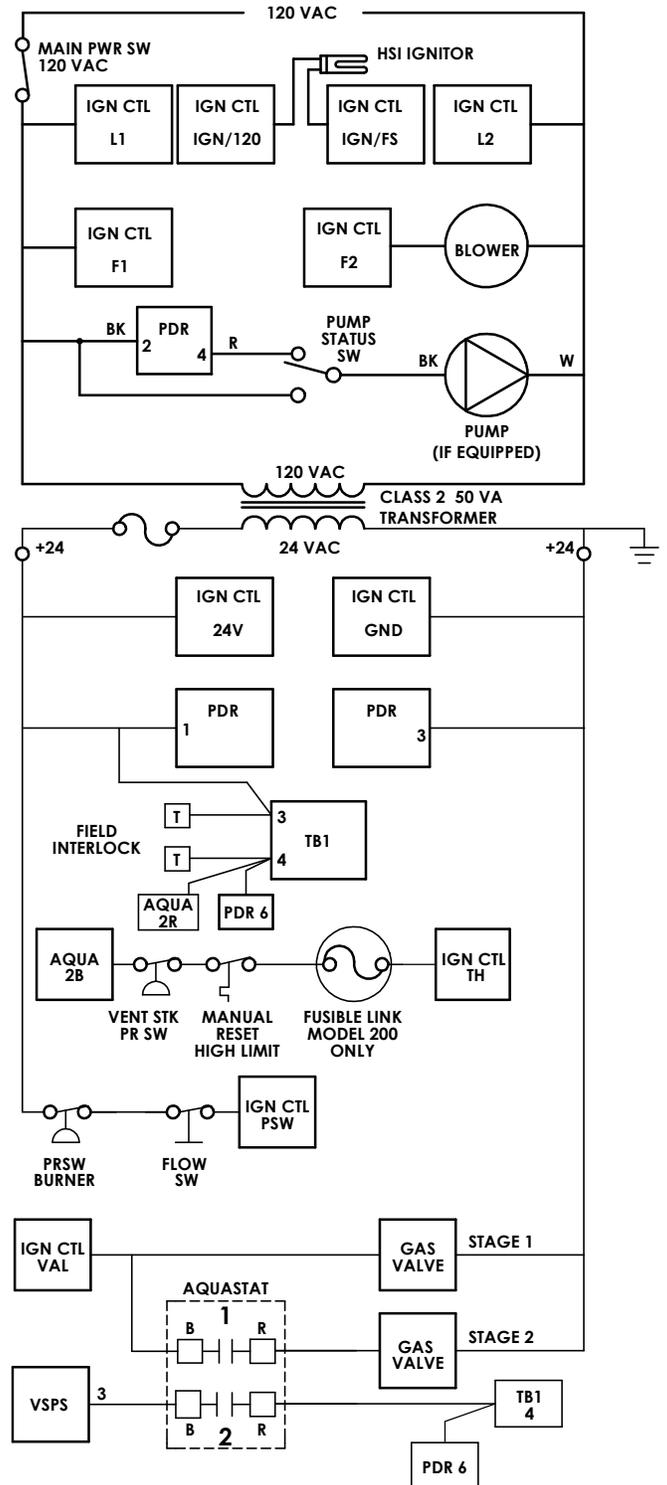
Figure 15. Logic Diagram, Volume Water Heater
