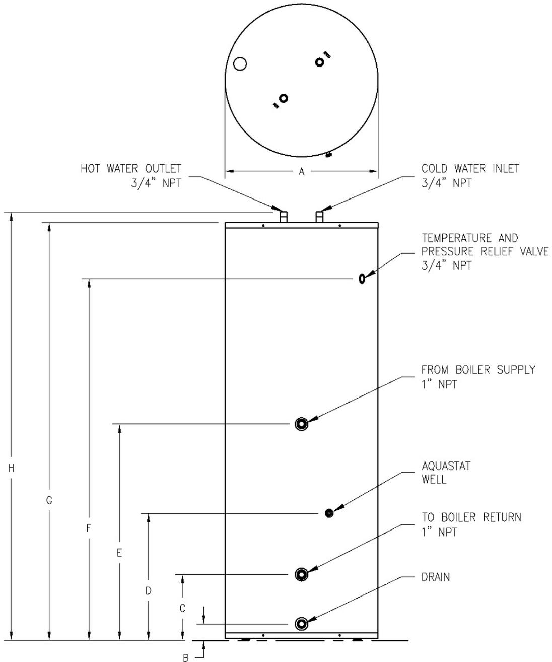
**Figure 1 – Heater Layout (30,40, 50, 75 single exchanger models)**
