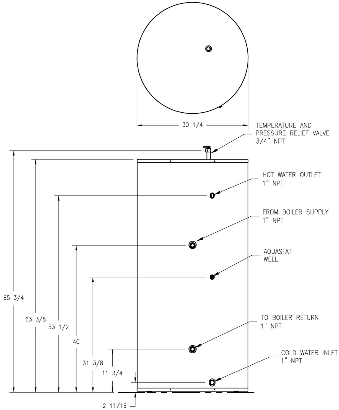
**Figure 2 – Tank Layout (120 gallon model)**
