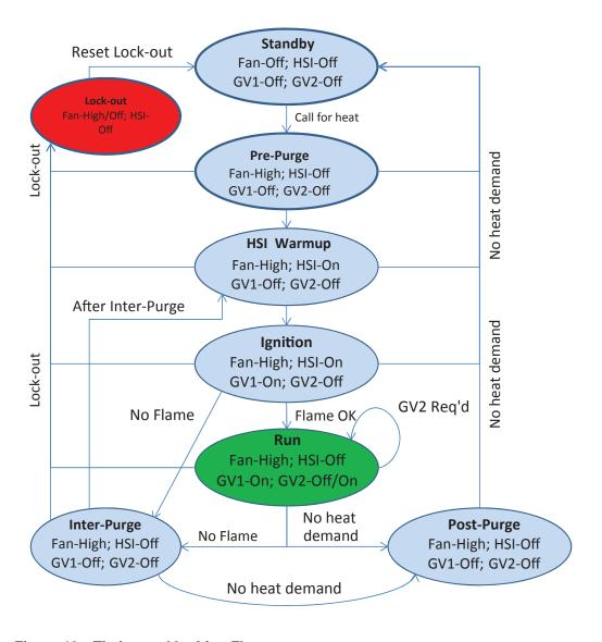
Figure 19. Timing and Ignition Flow
