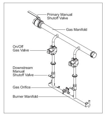
Figure 20. Typical Gas Train Configuration.
