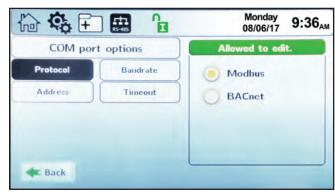
Screen 21. COM Port Config Screen, ModBus
