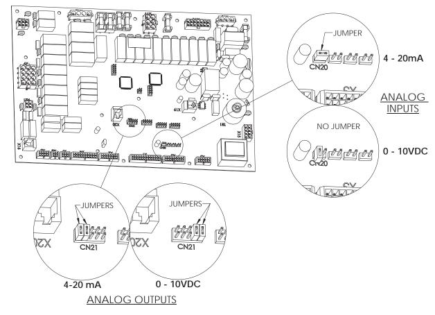
Figure 9. Analog Input and Output Jumper Placement
