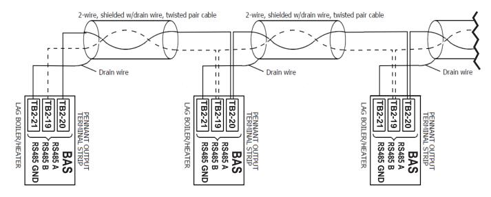
Figure 10. BAS Wiring Connections, Cascaded
