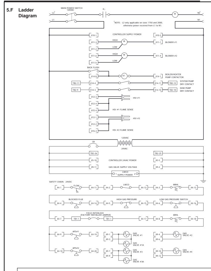
Figure 12. Ladder Diagram. Sizes 500 - 2000.
