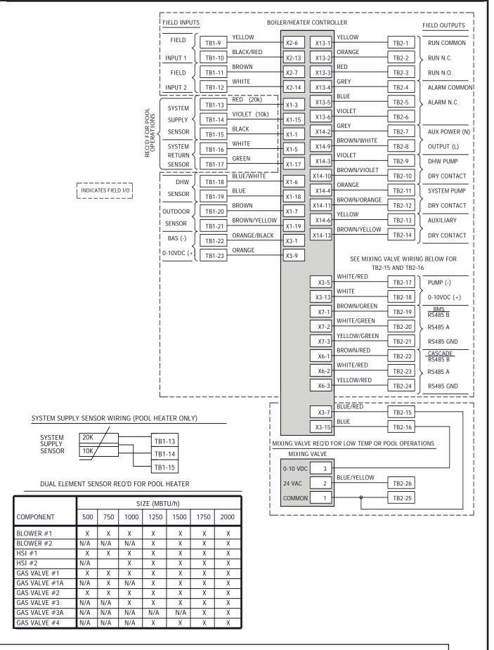
Figure 11. Wiring Diagram. Sizes 500 - 2000.
