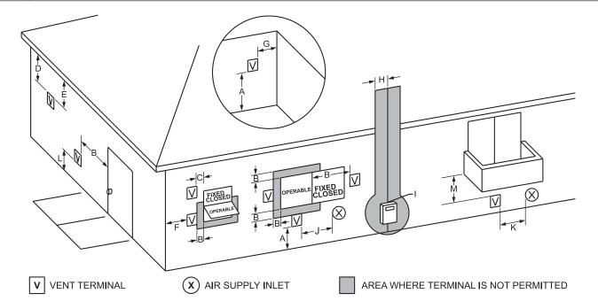
Figure 4. Combustion Air and Vent Through Side Wall.
