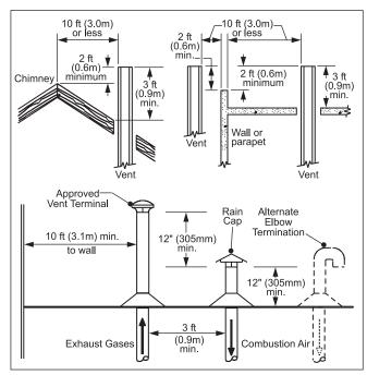
Figure 3. Combustion Air and Vent Through Roof.
