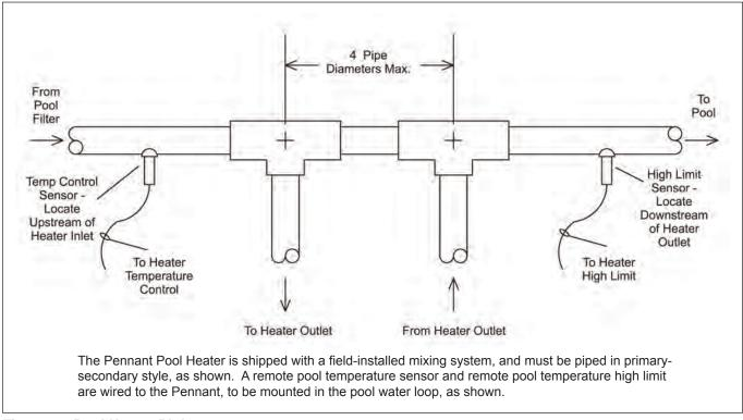
Figure 6. Pool Heater Piping.
