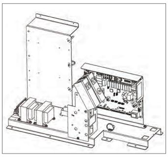
Figure 21. Typical Control Panel.
