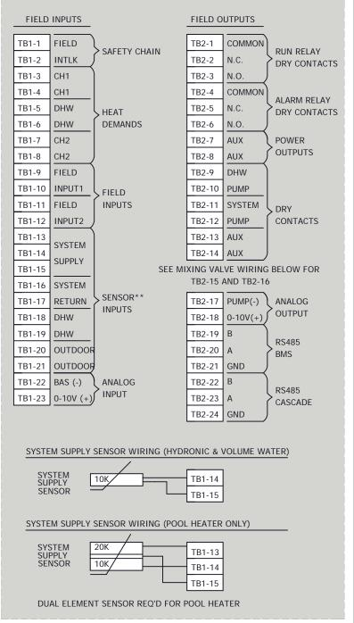
\*\*SYSTEM SUPPLY AND RETURN SENSORS ARE REQ'D FOR POOL OPERATIONS
