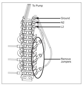
Figure 7. Removing Jumpers.
