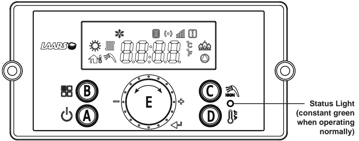
**The Control Display** has a Control Dial (E), 4 buttons (A, B, C, D), and a Liquid Crystal Display (with 72 back-lit segments). This section of this manual gives instruction on how to navigate into the many functions of the Mascot FT and to change temperature set points, set system variables and controller parameters.
