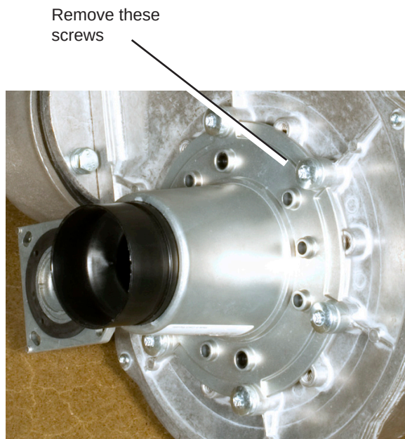
Fig. B23-8 - Separate the Venturi from the blower
