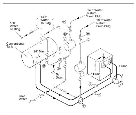
Figure 10. Safety-Flo Two Temperature Hot Water Supply System with Horizontal Tank.
