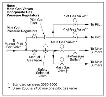
Figure 6. Typical Gas Piping Diagram.
