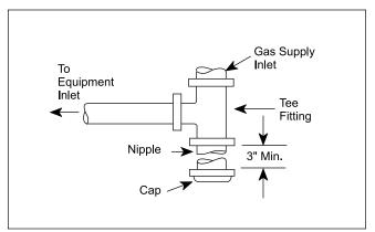
Figure 5. T-Fitting Sediment Trap Installation.
