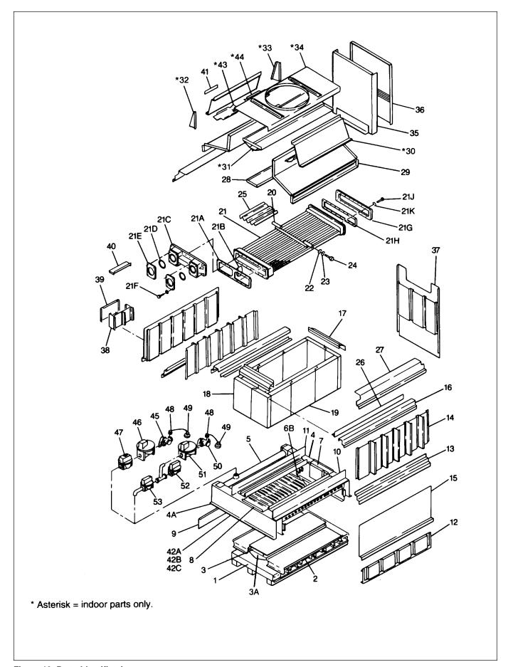
Figure 19. Parts Identification.
