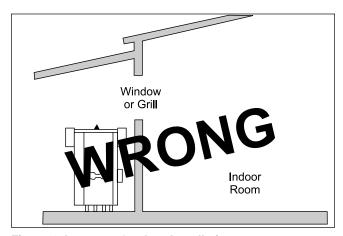
Figure 4. Incorrect Outdoor Installation.
