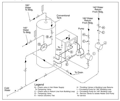
Figure 9. Supply-Flo Two Temperature Hot Water Supply System with Vertical Tank.
