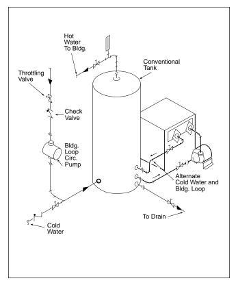
Figure 11. One Temperature Hot Water Supply System with Vertical Tank.
