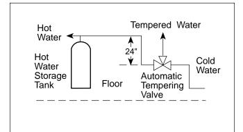
Figure 7. Tempering Valve Installation.
