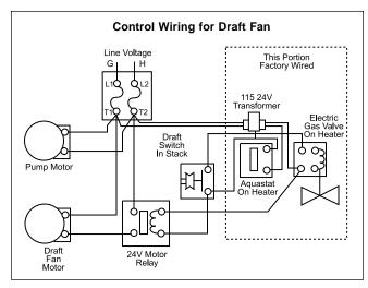
Figure 3. Draft Inducer/Power Venter.
