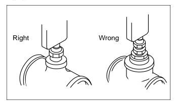
Figure 8. Thermometer Bulb.
