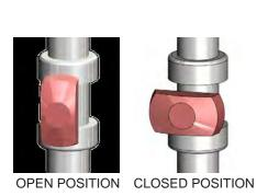
Figure 4. Gas Line Shut Off Valve
