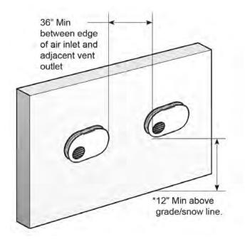
Figure 3. Multiple 2 pipe low profiles termination minimum spacings
