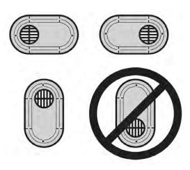
Figure 1. Possible orientations of low profile 2-pipe termination
