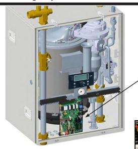
The DIP Switches are located at the bottom of the Printed Circuit Board (PCB). The PCB faces forward at the inside of the boiler. Remove the cover to locate the PCB.
