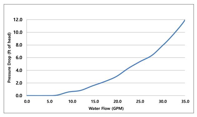
Figure 9. Water side pressure drop versus water flowrate for FT301 and FT399 Models
