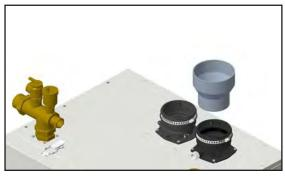
4" pipe connected, using a (3" to 4") adapter
