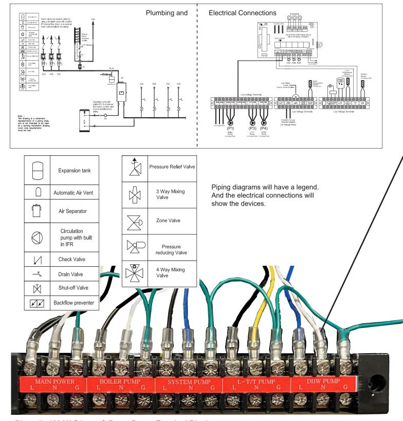
Photo 5. 120 VAC Input & Pump Power Terminal Block
