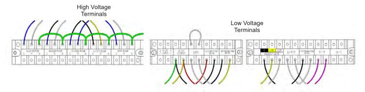
0-10 VDC Signal Input, 24 VAC Output, External LWCO, Cascade Sensor, DHW Sensor
