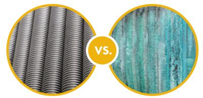
OmniTherm heat exchangers use 439 corrosion resistant stainless steel tubing that can withstand continuous operation in condensing conditions and remain in pristine condition. **Typical** vertical copper finned heat exchangers are prone to air side fouling after repeated exposure to condensing conditions. Poor combustion, reduced efficiencies and boiler failure can ultimately occur.
