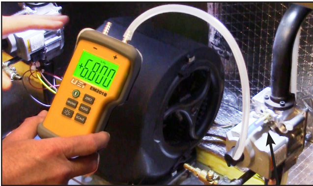
Figure 1. Measure Supply Gas Pressure
