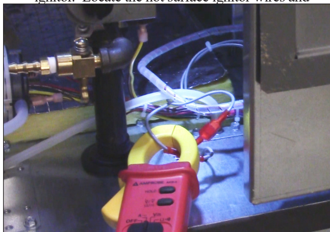
Figure 7. Amp Meter looped around an HSI wire.
