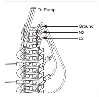
Figure 21. Removing Jumpers
