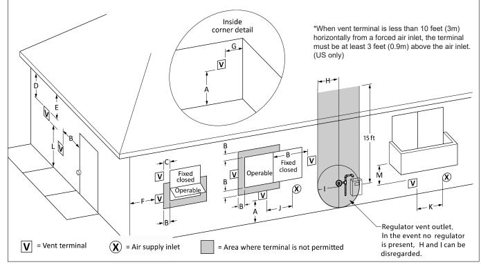
Figure 3. Combustion Air and Vent Through Side Wall.
