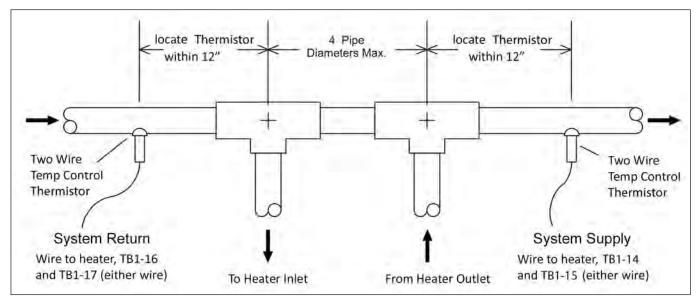
Figure 4. Low-Temp Heater Piping.
