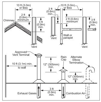
Figure 2. Combustion Air and Vent Through Roof.
