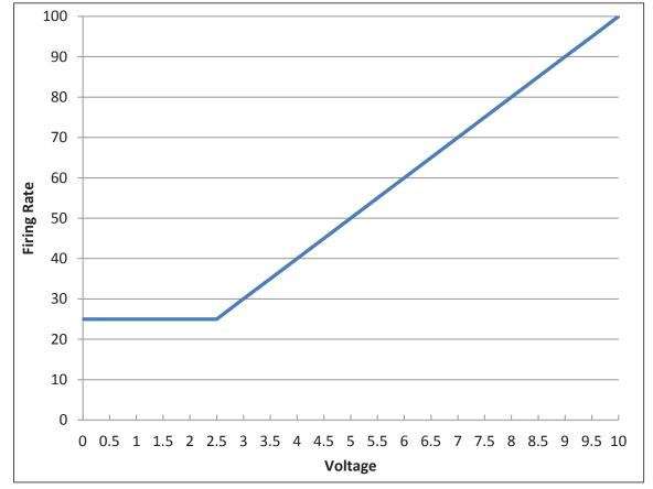
Figure 34. Firing Rate Control
