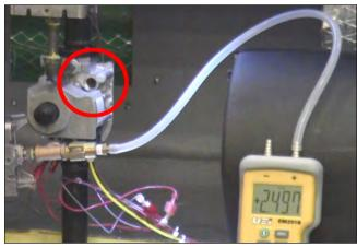
Figure 40. Measure/Adjust Manifold Pressure.
