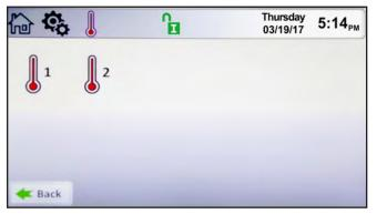
There are two identical heat demands, CH1 and CH2, each with independent control algorithms and independent inputs on the input terminal strip, see Figure 24 on page 36.
