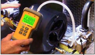
Figure 36. Measure Supply Gas Pressure
