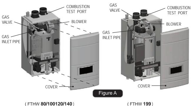
3. Using a Phillips screwdriver, remove the 4 screws on the front cover. See Figure A.
