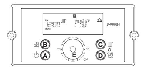
**To change Storage Mode Temp,** First turn OFF the power to the Control Display. Then Press and Hold Button B  $\blacksquare$  to get into the Installer Mode.
