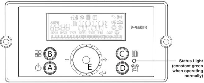
**The Control Display** has a Control Dial (E), 4 buttons (A, B, C, D), and a Liquid Crystal Display (with 72 back-lit segments). This section of this manual gives instruction on how to navigate into the many functions of the FT and to change temperature set points, set system variables and controller parameters.
