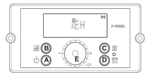
To change any of the Installer Parameters, Start by turning OFF the Power to the Display Control.
