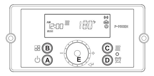
To change CH Setpoint, press the C button. The CH Icon and current CH Setpoint will flash.
