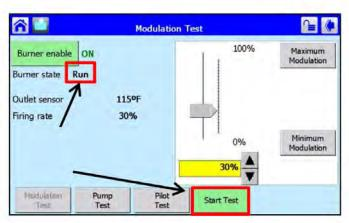
7. Confirm that the boiler is running and then press 'Start Test'
