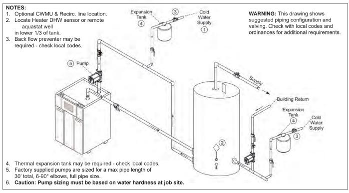
Figure 29. DHW Piping, One Heater, One Vertical Tank
