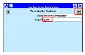
From the 'Warm Weather Shutdown' screen, adjust the setpoint.
