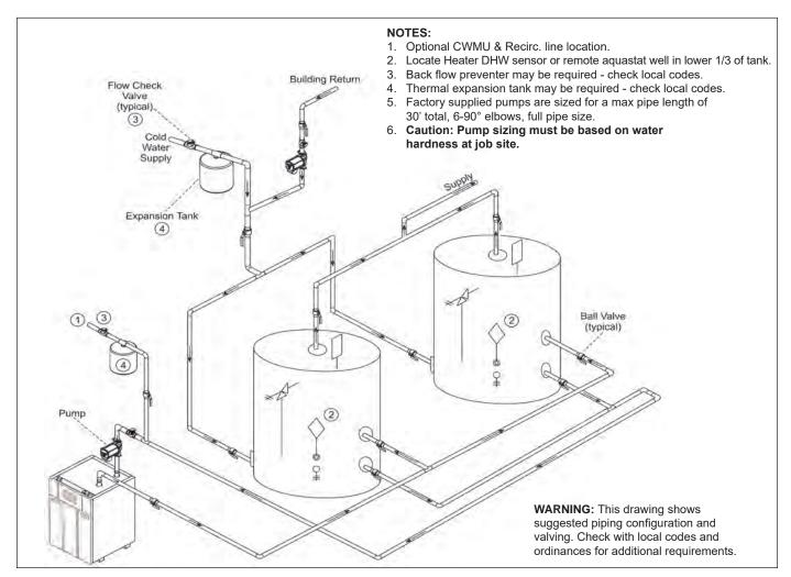
Figure 30. DHW Piping, One Heater, Two Vertical Tanks
