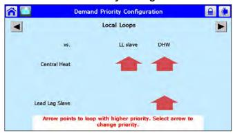
From the Demand Priority Configuration, the installer can adjust the priority of the different demand types. Central Heat, Lead Lag, Domestic Hot Water The control uses arrows as indicators to point to the loop with higher priority.
