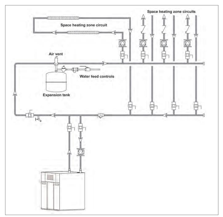
Figure 22. Hydronic Piping — Single Boiler, Zoning with Circulators
