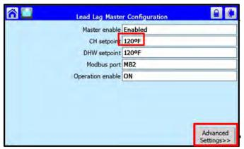
With the Master Control now Enable, press the setting box labeled 'CH setpoint'. Here you can adjust the desired Lead/ Lag system setpoint.
