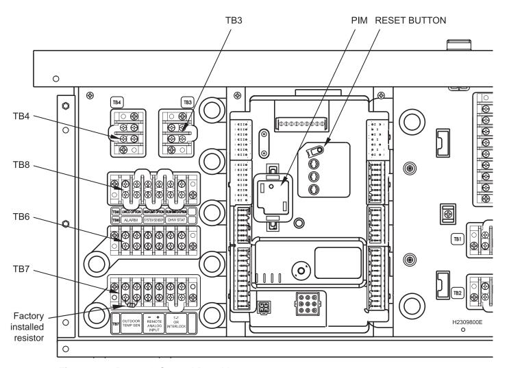
Figure 33. Power & Control Panel Layout
