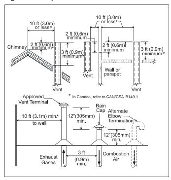
Figure 17. Combustion Air and Vent Through Roof
