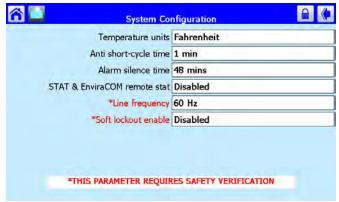
The installer can set the control to display temperature units in °F or °C, can adjust the anti short -cycle time, the low fire cutoff time, burner off inhibit time, and can set the time allowed for an alarm to sound before being silenced.
