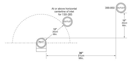
Figure 19. Minimum Venting Distance
