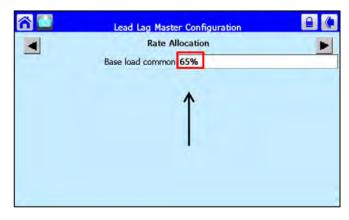
Adjust the "Base Load Common" value to the number of boilers in the cascade system. See chart for values.
