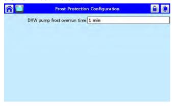
Frost protection will assist in keeping the unit from freezing when the unit is not able to fire, but is still able to run the pumps. The frost overrun time can be changed on this screen.
