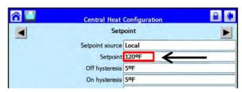
Press on the 'Setpoint' box to make adjustments to setpoint, and modulation for a single boiler CH demand.
