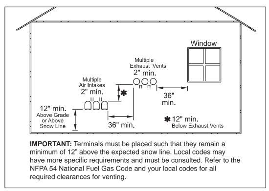
Figure 21. Multiple Side-Wall Terminals,
