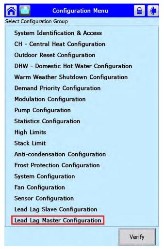
In the configuration menu, scroll down to the bottom and press onto Lead Lag Master Configuration.
