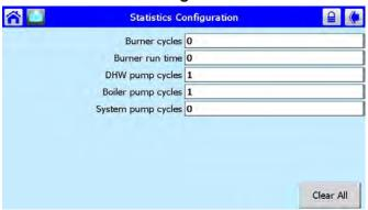
The statistics configuration sub-menu allows the installer to view Burner Cycles, Burner Run Time, DHW Pump Cycles, Boiler Pump Cycles, and System Pump Cycles.
