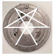
Figure 48. Torque Pattern
