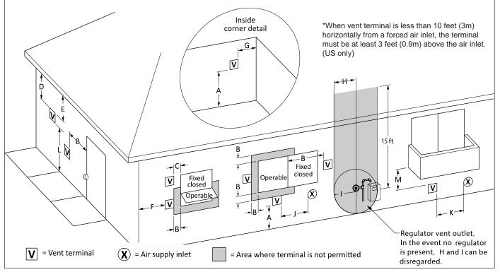
Figure 20. Combustion Air and Vent Through Side Wall
