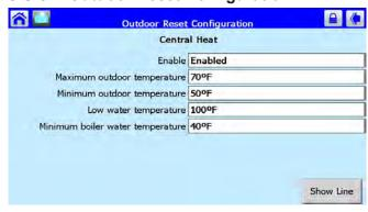
At this sub-menu, confirm that Central Heat is Enabled. Next, press onto the Maximum Outdoor Temperature, Minimum Outdoor Temperature, and Low Water Temperature to get to each and adjusting their setpoints in those sub-menus.
