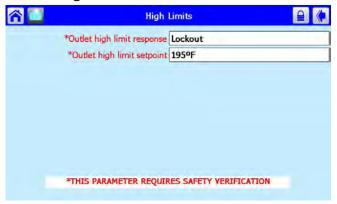
The outlet High limit can be adjusted using the installer password. After a change is made, the control will lockout and require a Safety Verification (see Section 8.3 for more details on Safety Verification).
