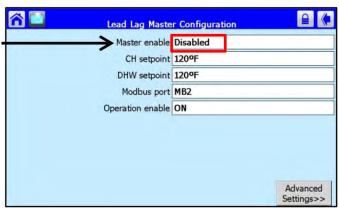
Confirm the Master control is 'Enabled'. If not enabled, press to select.
