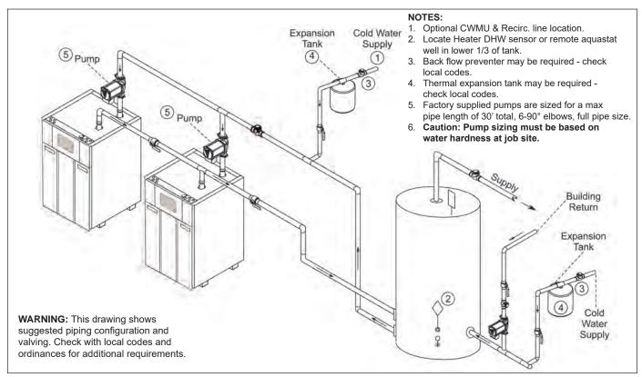
Figure 31. DHW Piping, Two Heaters, One Vertical Tank
