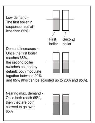
Figure 40. Lead Lag Operation, 2 boilers.
