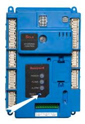
Figure 39. Reset Button on Controller
