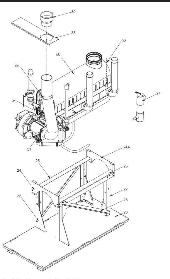
Parts Illustration 5. Internal Components, Sizes 750-850
