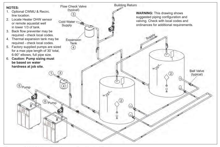
Figure 32. DHW Piping, Two Heaters, Two Vertical Tanks
