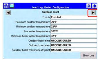
If you are using Outdoor Reset for Lead/ Lag, adjust the Maximum Outdoor Temp, Minimum Outdoor Temp and Low Water Temp by touching each set point line. The set point screen will appear. Make the adjustment, then press OK.
