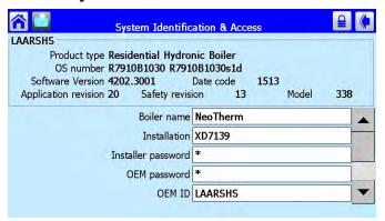
This sub-menu will display information regarding software, date codes, model numbers and program name, as well as giving the installer access to re-name the boiler and to change the modbus addresses for lead lag operation. Press the back arrow on the top right corner of the screen to return to the 'Configuration Menu'.
