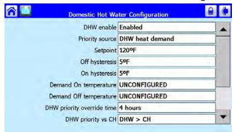
DHW - Domestic Hot Water is used to configure the DHW temperature parameters for water heaters (Heater) and for indirect water heaters that are used with boiler (Boiler) systems.
