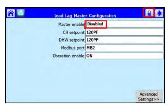
Make sure that Master enable is 'Disabled' then press the Back arrow to return to the configuration menu. Then you will need to confirm that the Follower configuration is **Enabled**.
