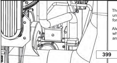
The Gas Valve in the **399 and 500** is at the front of the unit and can be reached after the front panel is pulled forward and then off.
