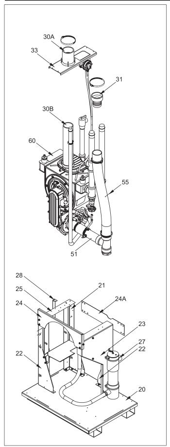
Parts Illustration 3. Internal Components, Sizes 150–199
