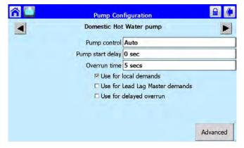
The DHW pump connections are located on terminal block 5 (TB5) in the control panel and are rated for 120Vac, 7.4 Amps. To use the contacts, power must be supplied on one terminal, and the other terminal wired to the pump or a relay controlling the pump. Additional 120VAC circuits may be required for the pumps.
