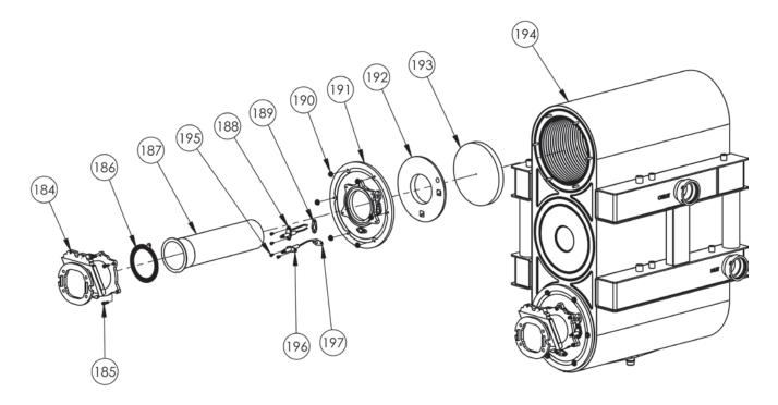
Fig. 147 - Heat Exchanger Components
