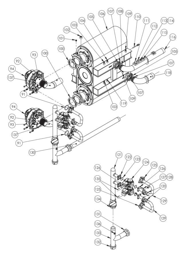
Fig. 145 - Burners and Combustion Chamber
