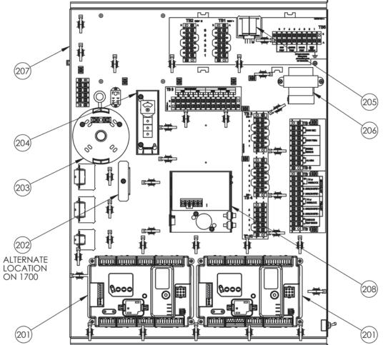
Fig. 150 - Electronic Components
