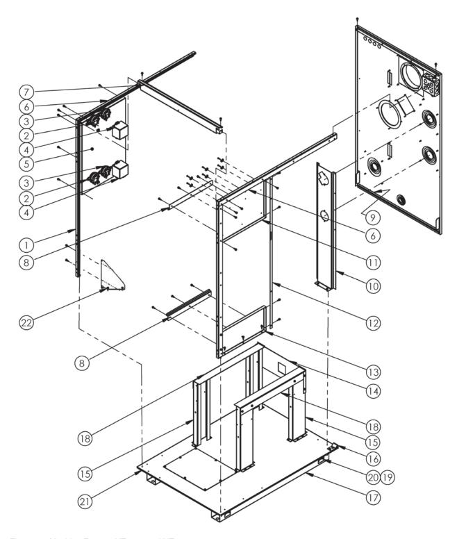
Fig. 140 - Machine Frame - NT1000 and NT1200
