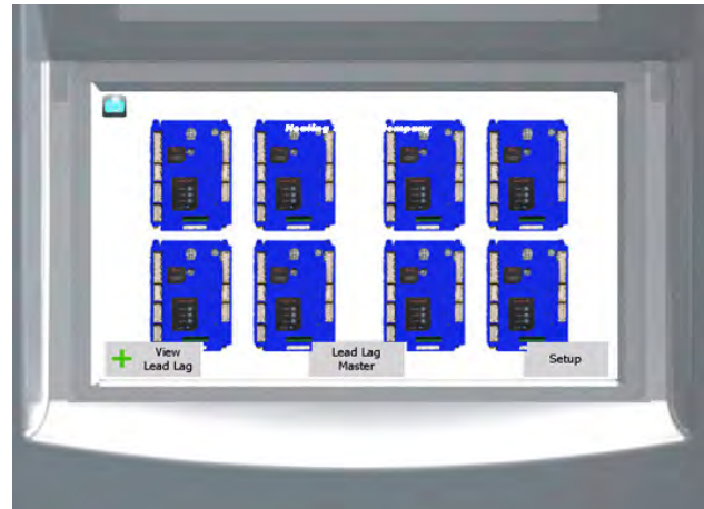
Figure 26. Touch Screen, shown with the 'home' screen of the lead boiler in a four boiler configuration, all conditions normal.
