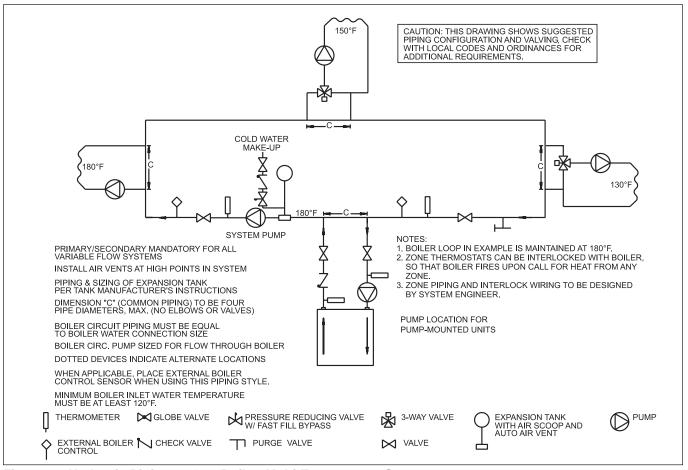
Figure 7. Hydronic Piping — One Boiler, Multi-Temperature System.
