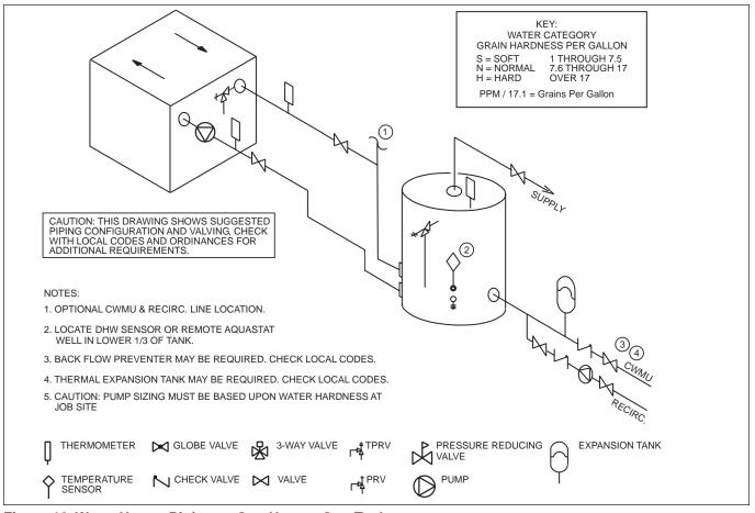
Figure 10. Water Heater Piping — One Heater, One Tank.
