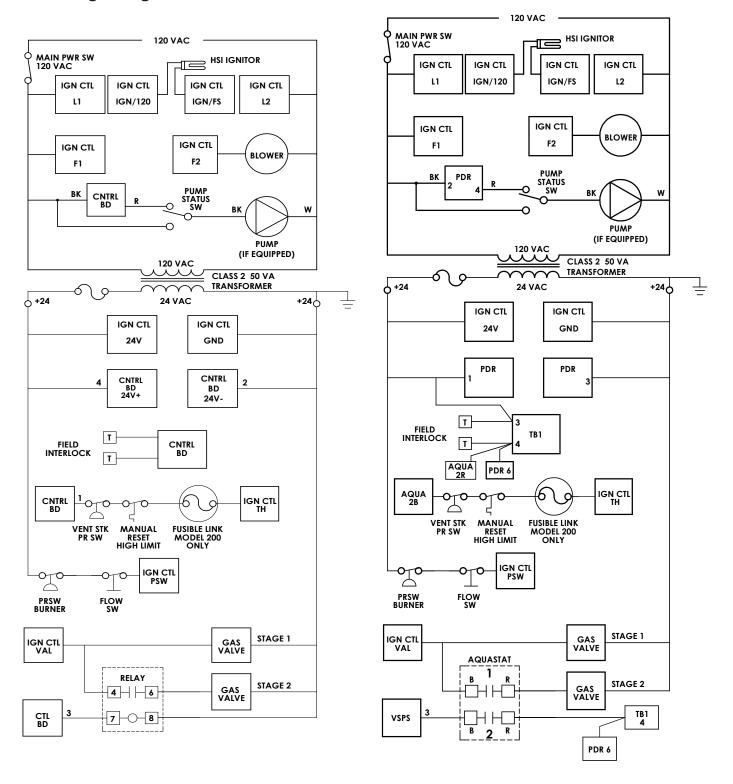
Figure 14. Logic Diagram, Hydronic Boiler
