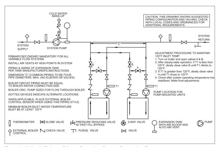
Figure 9. Hydronic Piping — Primary-Secondary, Reverse-Return, Low Temperature.
