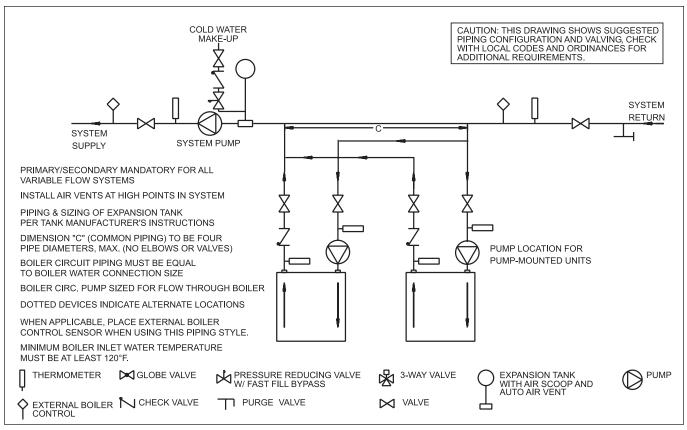
Figure 8. Hydronic Piping — Primary-Secondary, Reverse-Return.
