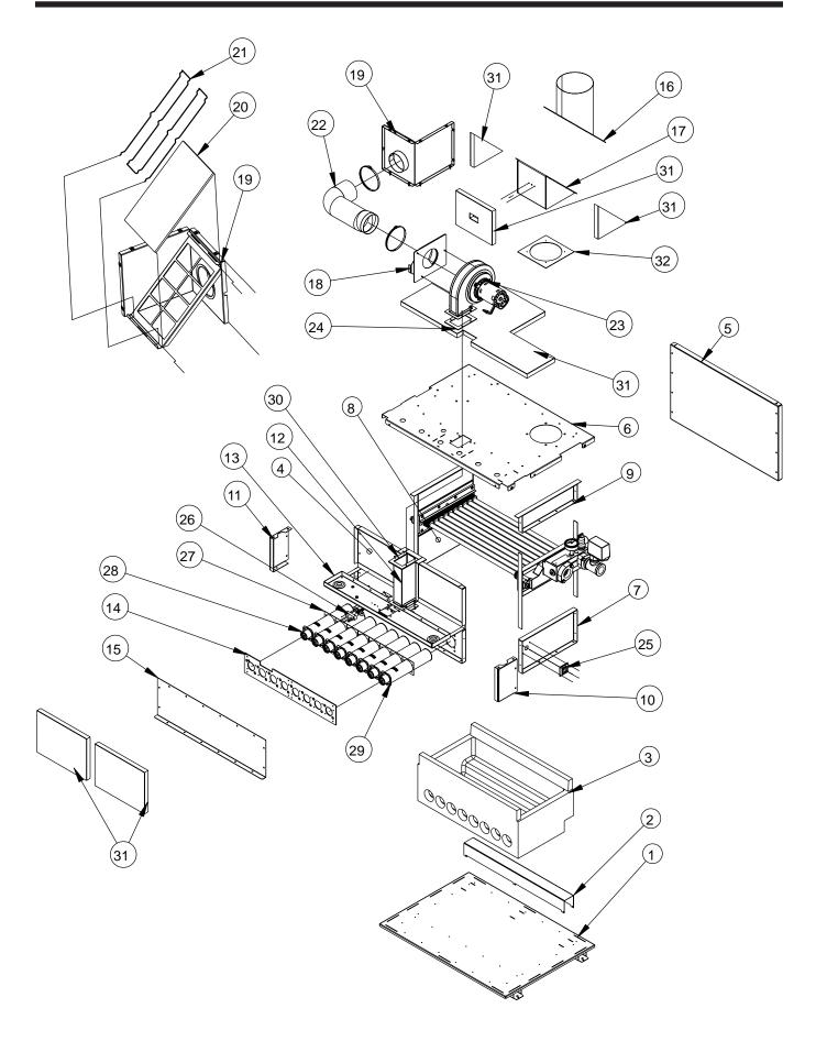
Figure 19. Combustion Chamber Components.
