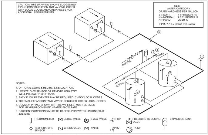
Figure 13. Water Heater Piping — Multiple Heaters, Multiple Tanks.
