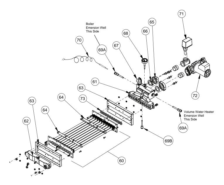
Figure 21. Heat Exchanger Components.
