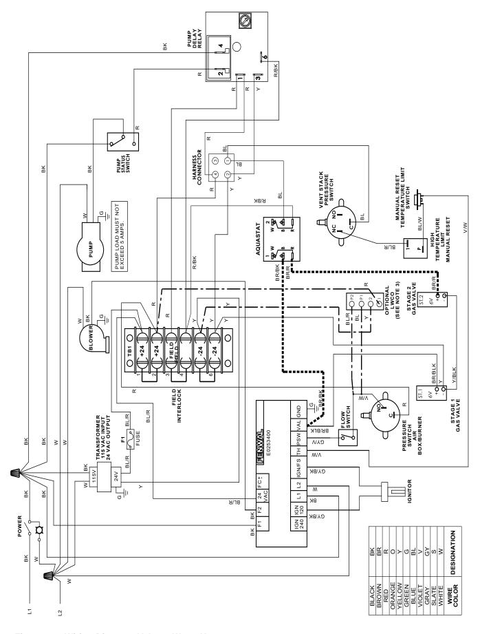
Figure 17. Wiring Diagram, Volume Water Heater.
