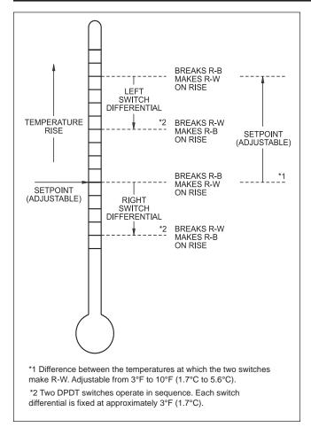
Figure 18. Two stage aquastat
