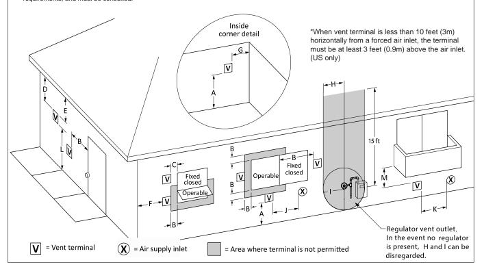
Figure 4. Vent Terminal Clearance.
