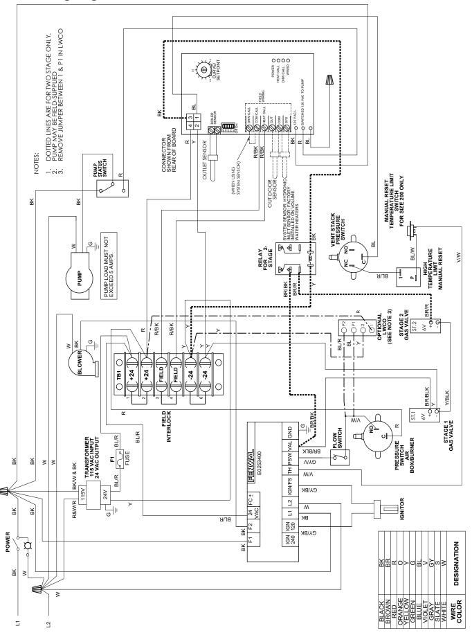
Figure 16. Wiring Diagram, Boiler.
