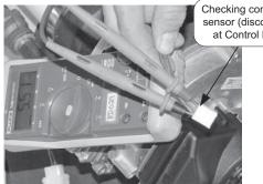
Checking continuity of sensor (disconnected at Control Board)
