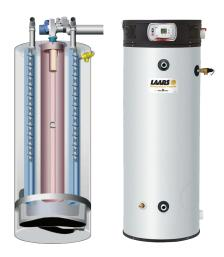
Three Pass Heat Exchanger System—The three pass Heat Exchanger system keeps the hot combustion gases moving at a high velocity. The combination of high turbulence and velocity causes an enormous rate of heat transfer into the water.
