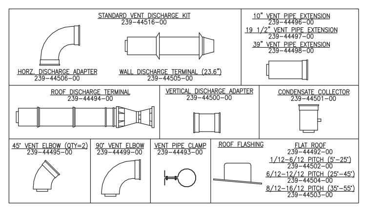
Note: When ordering service replacement parts, the full model and serial numbers from the water heater nameplate are required.
